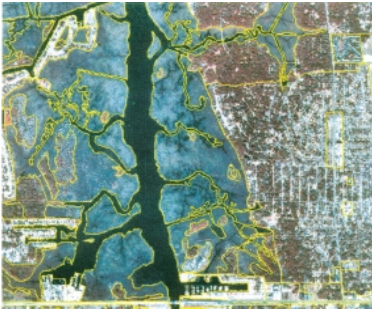
Figure 1 Digitized National Aerial Photography Program (NAPP) image (1 x 1 m) of Jacksonville Beach, FL with vectors derived from “on-screen” visual image interpretation.
