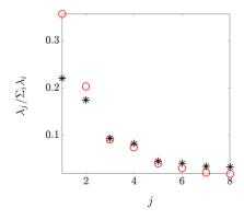
FIG. 17. Contribution of the first eight eigenvalues of the velocity covariance matrix  $\Phi$  of channel flow in the absence (\*), and presence (o) of base flow perturbations with  $f(y) = \bar{U}(y)/\max(|\bar{U}(y)|)$  and amplitude  $\alpha = 1$  in turbulent channel flow with  $R_{\tau} = 186$  at  $(k_x, k_z) = (1.86, 1.94)$ .
