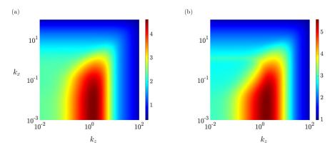
FIG. 6. Energy spectra of (a) plane Couette flow with R = 500 and (b) plane Poiseuille flow with R = 2000. Color plots show  $\log_{10}[E_0(\mathbf{k})]$ .
