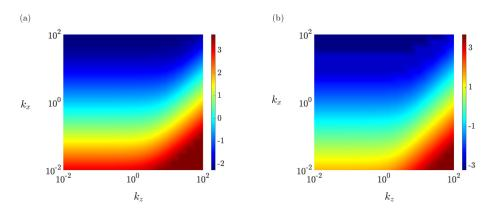
FIG. 5. Logarithmically scaled critical variance levels for stochastic multiplicative uncertainty  $\bar{\gamma}_u$  with  $\alpha=1$  and  $f(y)=\bar{U}(y)/\max(|\bar{U}(y)|)$  over the horizontal wavenumber spectrum in (a) Couette flow with R=500 and (b) Poiseuille flow with R=2000.
