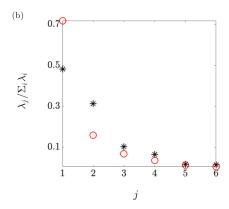
FIG. 11. Contribution of the first six eigenvalues of the velocity covariance matrix  $\Phi$  of channel flow in the absence (\*) and presence ( $\circ$ ) of base flow perturbations with  $f(y) = \bar{U}(y)/\max(|\bar{U}(y)|)$  and amplitude  $\alpha = 1$ . (a) Couette flow with R = 500 at  $\mathbf{k} = (0.95, 2.29)$ ; and (b) Poiseuille flow with R = 2000 at  $\mathbf{k} = (0.38, 3.02)$ . The variance of base flow uncertainties: (a)  $\sigma_u^2 = 0.50$ ; (b)  $\sigma_u^2 = 0.21$ .
