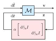
FIG. 3. Linear fractional transformation of an LTI system subject to both additive and multiplicative stochastic disturbances [Eqs. (12)]. Here,  $d\tilde{t}$ ,  $d\tilde{\gamma}_u$ , and  $d\tilde{\gamma}_w$  represent differentials of Wiener processes that model additive and multiplicative sources of stochastic uncertainty.
