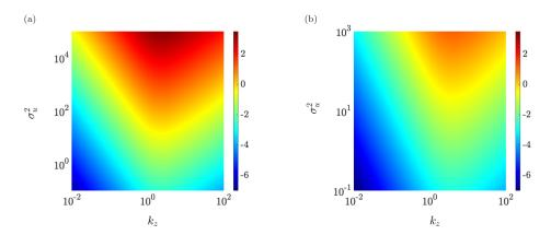
FIG. 20. Logarithmically scaled terms that are responsible for the  $O(R^2)$  energy amplification in Eq. (29)  $(\log_{10}[g(k_z,\sigma_u^2)])$  as a function of spanwise wavenumber  $k_z$  and base flow perturbation variance  $\sigma_u^2$ . Perturbations to the base flow follow  $f(y) = \bar{U}(y)/\max(|\bar{U}(y)|)$ . (a) Couette flow with R = 500; and (b) Poiseuille flow with R = 2000.
