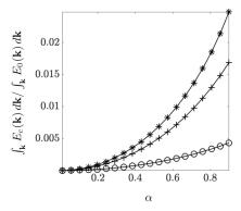
FIG. 16. The total effect of stochastic perturbations of amplitude  $\alpha$  on the energy spectrum of turbulent channel flow with  $R_{\tau} = 186$ . The curves demonstrate the  $\alpha$  dependence of the energy correction due to base flow perturbations entering the dynamics through the shape functions f(y) corresponding to Eq. (7) (+), in addition to those depicted in Figs. 2(a) (\*) and 2(b) ( $\circ$ ).
