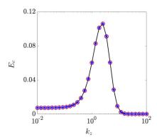
FIG. 7. The discounted energy spectrum  $E_c$  in Couette flow with R=500 and  $k_x=1$  subject to base flow perturbations with  $f(y)=\bar{U}(y)/\max(|\bar{U}(y)|)$  with  $\sigma_u^2=0.43$  and  $\alpha=0.01$ . Direct solution from solving Eq. (20) (–); and approximate solutions from perturbation analysis:  $E_c=\alpha^2 E_2(\mathbf{k})$  (\*) and  $E_c=\alpha^2 E_2(\mathbf{k})+\alpha^4 E_4(\mathbf{k})$  (o).
