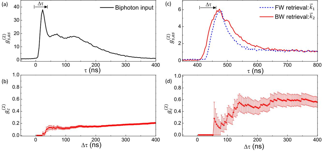
FIG. 3. Autocorrelation of a single-photon wave packet measured by a BS. (a) Incident anti-Stokes photon wave form and (b) its autocorrelation  $g_c^{(2)}$  measured with a conventional BS as a function of the coincidence time window length  $\Delta\tau$ . (c) Retrieved anti-Stokes photon wave form and (d) its autocorrelation  $g_c^{(2)}$  measured with the atomic BS.
