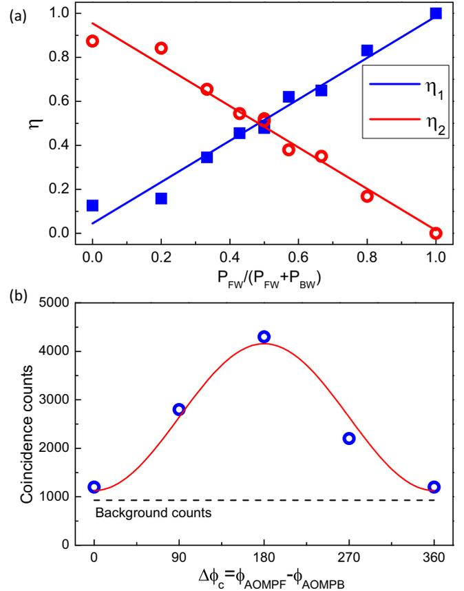
FIG. 4. (a) BS's FW and BW splitting ratios as functions of the FW control laser power. (b) Single-photon MZ interference result by varying the AOM-pair phase difference. The coincidence counts are measured over a 200-ns coincidence time window and total time of 300 min.
