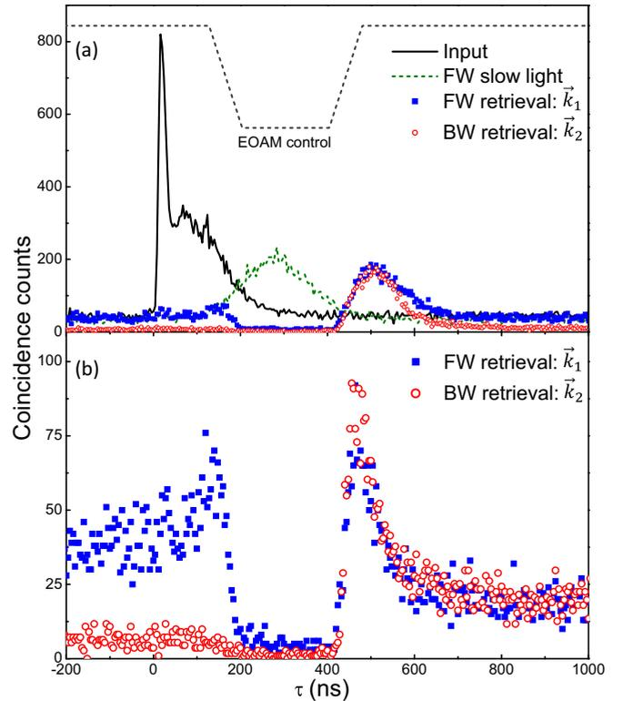
FIG. 2. Photon wave forms after the atomic BS measured as coincidence counts in 35 min with 4-ns time bin width. (a) FW or BW storage retrieval when only one retrieval (FW or BW) control beam is present. (b) BS output wave forms when both FW and BW retrieval control beams are present simultaneously.
