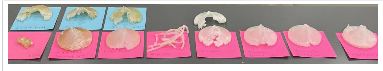
Figure 35 – Process changing injection parameters to achieve final product
