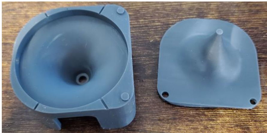
Figure 5 – Example 3D Printed Mold designed by peer Chase Pearson
