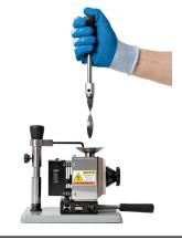
Galomb, Inc. 523 N 22<sup>nd</sup> Street Allentown, PA 18104 USA Ph (610) 434-3283 Fax (610) 434-1668 Website: <u>www.injectionmolder.net</u> Email: inquiry@injectionmolder.net Move the melt chamber to the Model-S machine and make an injection molded part with the mixed material.
