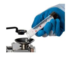
Melt the resin pellets and then mix materials with mixing tool.
