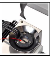
The helical mixing blade creates excellent laminar and chaotic flow within the melt chamber, allowing the entire melt to experience a uniform processing history.
