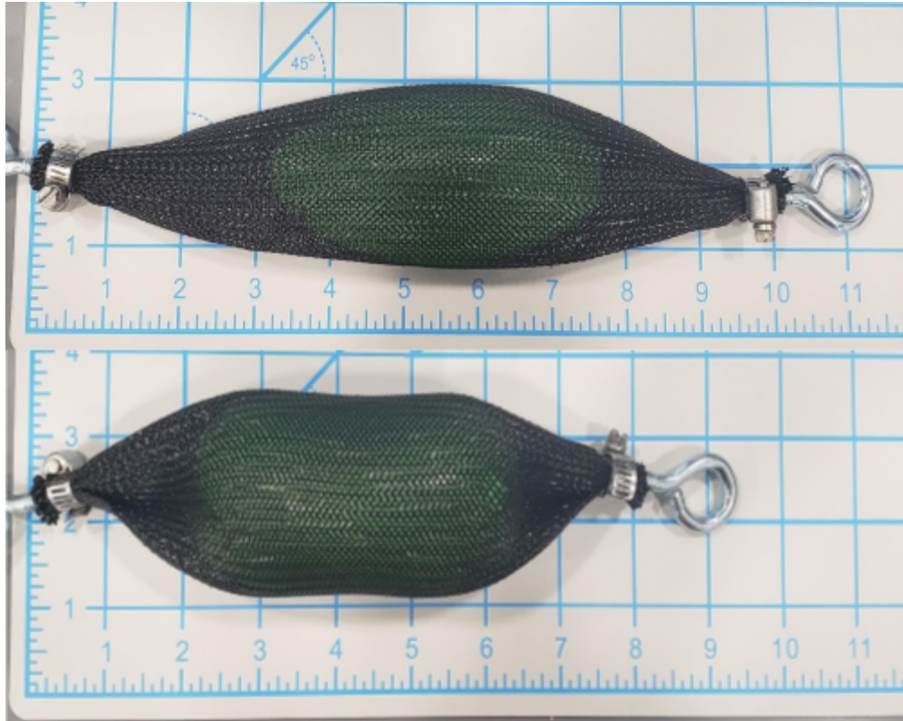
Figure 7. (Top) The pneumatic McKibben at its relaxed/expanded state and (Bottom) its contracted state
