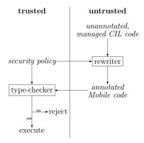
Figure 1.3: A Mobile load path
