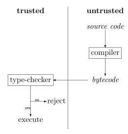
Figure 1.2: Bytecode type-checking
