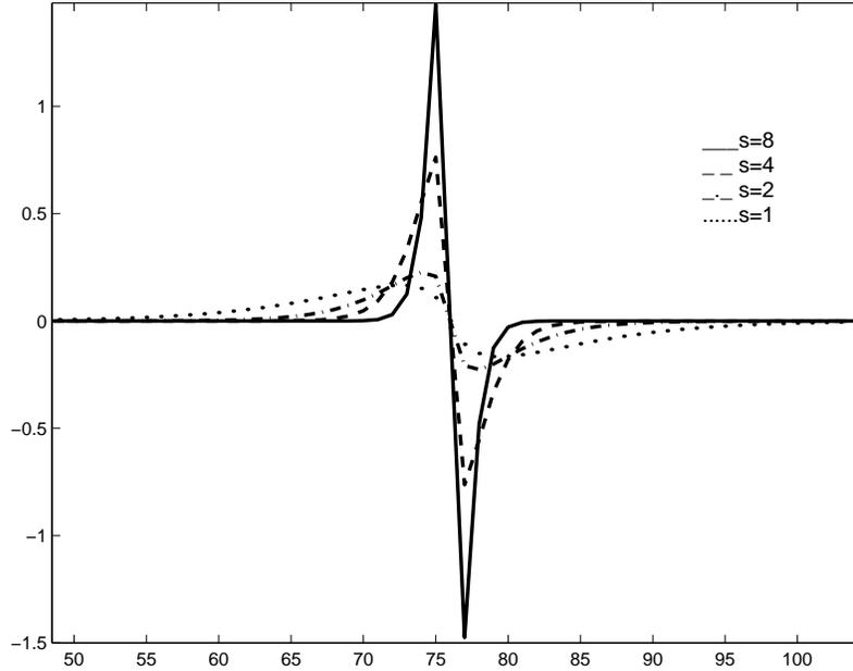
Figure 2: Impulse response of optimized Canny-Derliche filter for different scales.
