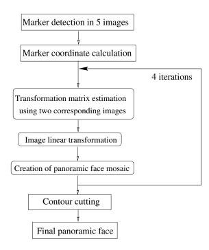
Figure 3. Block diagram of proposed panoramic face construction algorithm.
