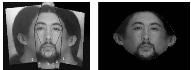
Fig. 9. Mosaicing results: Panoramic face composition from 5 views (left), and final mosaic (right).
