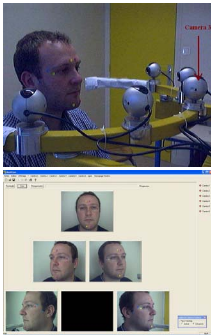
Fig. 1. The Acquisition system: the top panel shows the 5 cameras and their support, the bottom panel shows the five images collected from a subject. Each image size is 240 \times 320 pixels.
