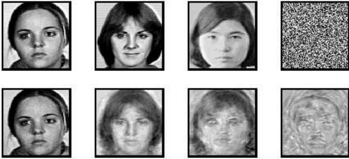
FIG. 4. — The top panels show four stimuli presented as memory keys and the bottom panels the responses produced by an autoassociative memory trained with 160 Caucasian faces. From left to right the stimuli are 1) a Caucasian face that has been learned by the memory, 2) a Caucasian face that has not been learned by the memory, 3) a Japanese face that has not been learned by the memory, and 4) a random pattern. The learned face is reconstructed perfectly by the memory ( r^2 = 1 ). The Japanese face is more distorted by the memory than the new Caucasian face ( r^2 = .72 vs .82 , respectively) and the random vector becomes less and less face-like ( r^2 = .00 ).
