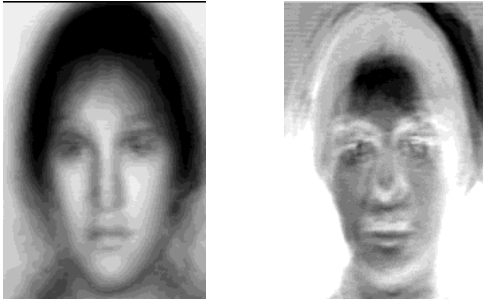
FIGURE 9. The first two eigenvectors of an autoassociative memory created from 25 male and 25 female face images.
