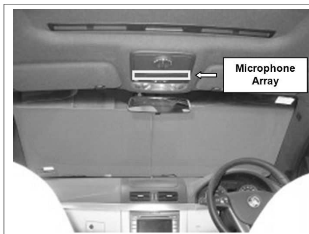
Figure 4.1: Location of 8-microphone array used in collecting the Australian English In-Car Speech corpus.
