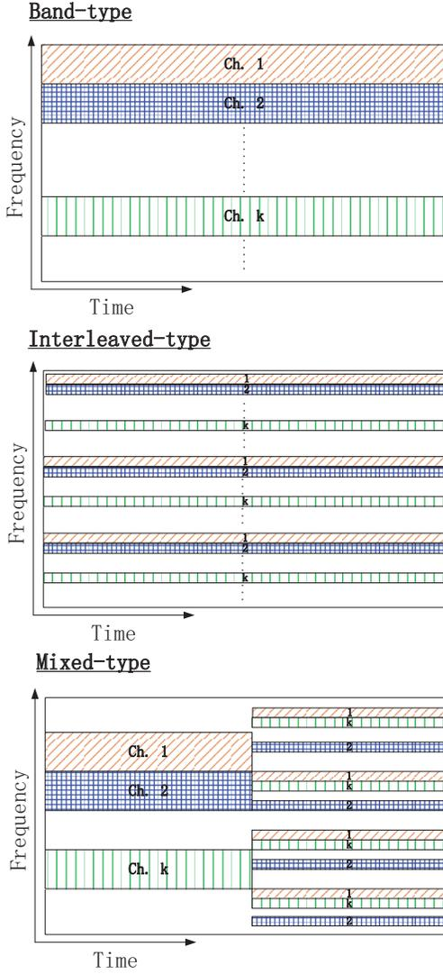
Fig. 1. Alternative subchannel structures
