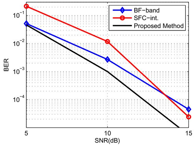
Fig. 4. BER performance for 16-QAM modulation with rate 1/2 convolutional code,  $n_t=2$ ,  $n_r=1$ , mobile speed=200km/h.
