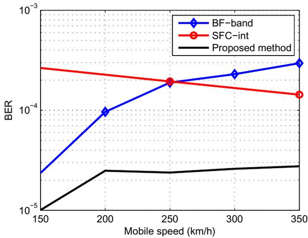
Fig. 3. BER performance for 16-QAM modulation with rate 1/2 convolutional code,  $n_t=4$ ,  $n_r=1$ , SNR=8dB.
