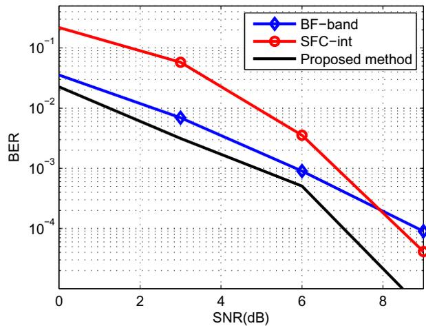
Fig. 5. BER performance for 16-QAM modulation with rate 1/2 convolutional code,  $n_t=4$ ,  $n_r=1$ , mobile speed=250km/h.
