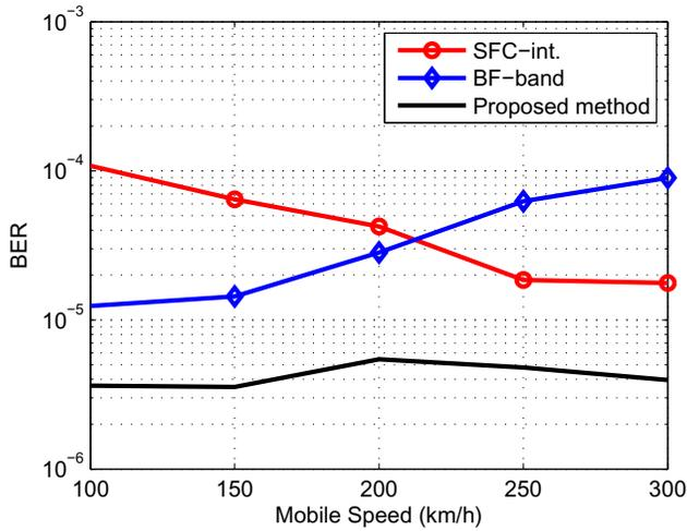
Fig. 2. BER performance for 16-QAM modulation with rate 1/2 convolutional code,  $n_t=2$ ,  $n_r=1$ , SNR=15dB.
