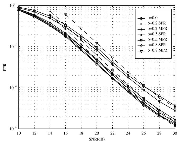
Fig. 2. FER simulation performance (solid line) of DSTBC with BPSK, at fading rate 0.01, cross correlation = 0.0, 0.2, 0.5, 0.8, with SPR and MPR receivers, and corresponding upper bounds of MPR (dash lines).
