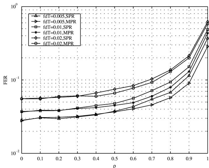
Fig. 1. FER simulation performance of DSTBC with BPSK for different spatial correlation values, at SNR = 20 dB, with SPR and MPR receivers.
