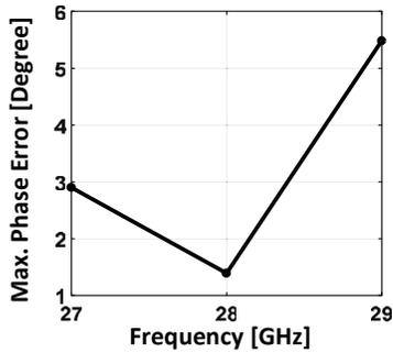
Fig. 8. Maximum phase error among output phases
