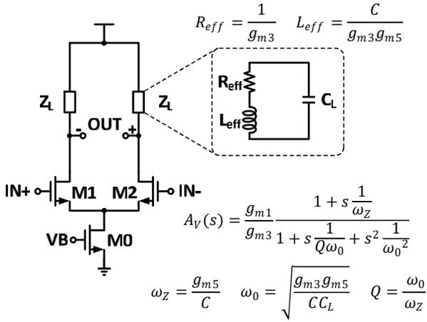
Fig. 3. Delay unit equivalent circuit
