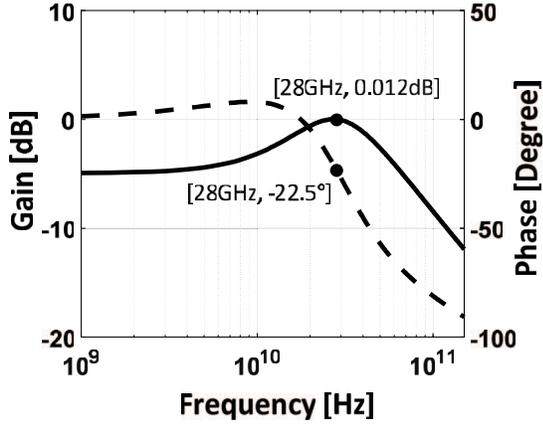
Fig. 4. Simulated delay unit frequency response
