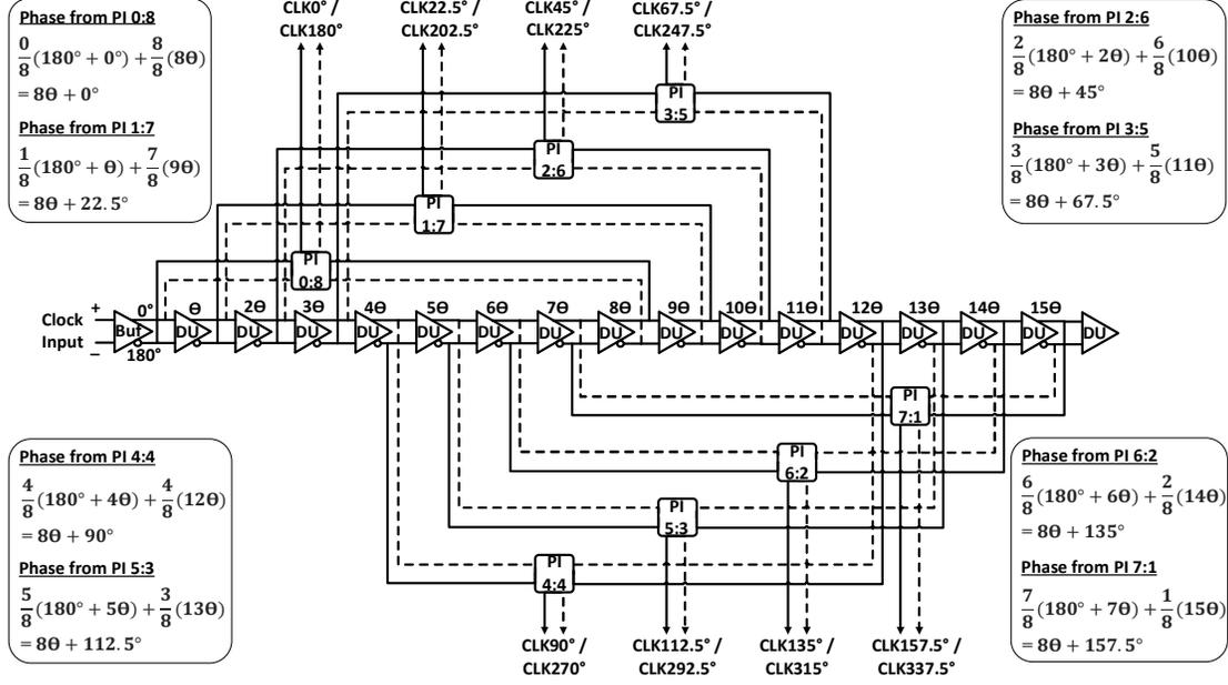
Fig. 1. The architecture of the open-loop 16-phase differential clock generator
