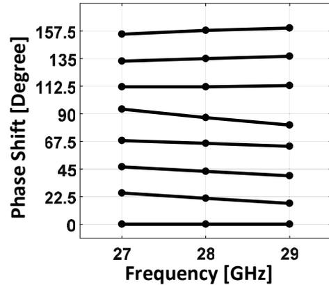
Fig. 7. Phases of the multi-phase clock outputs
