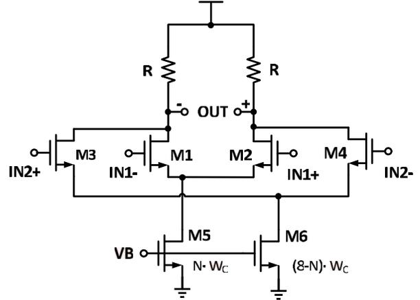
Fig. 5. Phase interpolator
