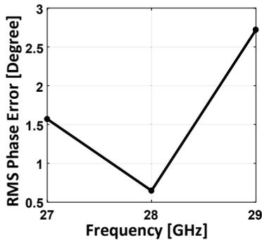
Fig. 9. RMS phase error among output phases
