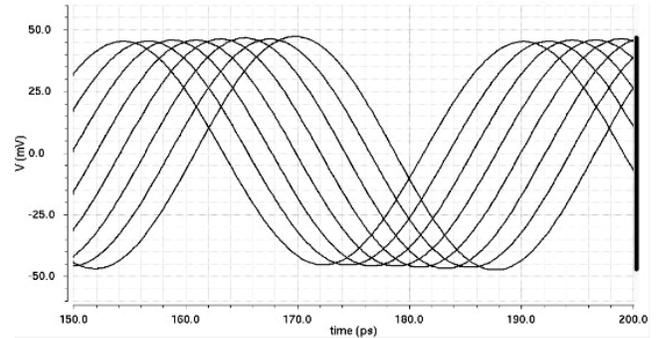
Fig. 6. Multi-phase clock generator outputs.
