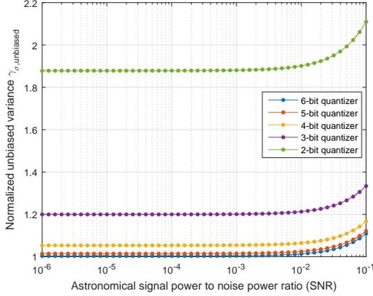
Fig. 4. Performance of normalized variance of RAS signal power estimation after the bias compensation ( $\sigma_s^2 = 1$ ,  $N$  or  $L = 10^4$ )
