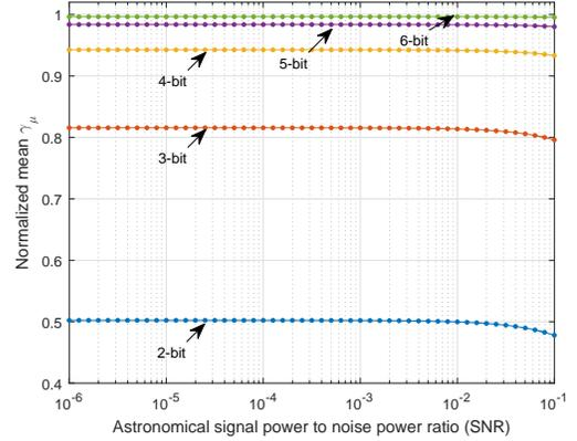
Fig. 2. Performance of normalized mean of RAS signal power estimation under various ADC resolutions ( $\sigma_s^2 = 1$ ,  $N$  or  $L = 10^4$ )
