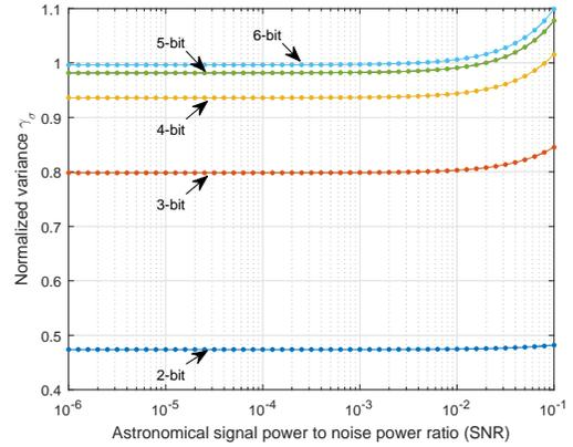
Fig. 3. Performance of normalized variance of RAS signal power estimation under various ADC resolutions ( $\sigma_s^2 = 1$ ,  $N$  or  $L = 10^4$ )
