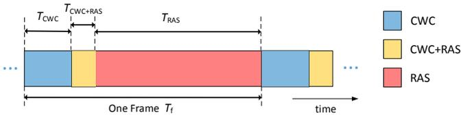
Fig. 1. Frame structure of the three-phase spectrum sharing paradigm where the durations of the phases could be different at different hours [10]
