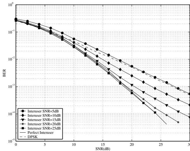
Fig. 4. BPSK differential modulation with incremental relaying protocol at various interuser SNRs
