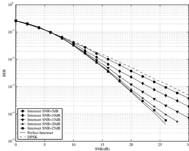
Fig. 3. BPSK differential modulation with selection relaying protocol at various interuser SNRs
