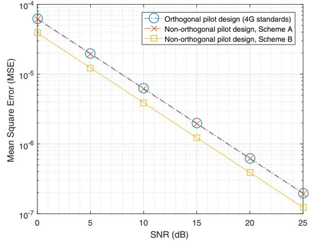
Fig. 8. Channel estimation performance for different pilot designs in the fractional bandwidth allocation
