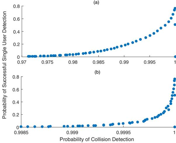
Fig. 6. Single user detection performance versus collision detection performance for different detection threshold values. a) 2 users per pilot group, b) 3 users per pilot group.
