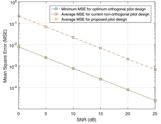
Fig. 3. Channel estimation performance comparison among different pilot designs in a system with  $N = 128$  subcarriers and  $L = 8$  channel taps
