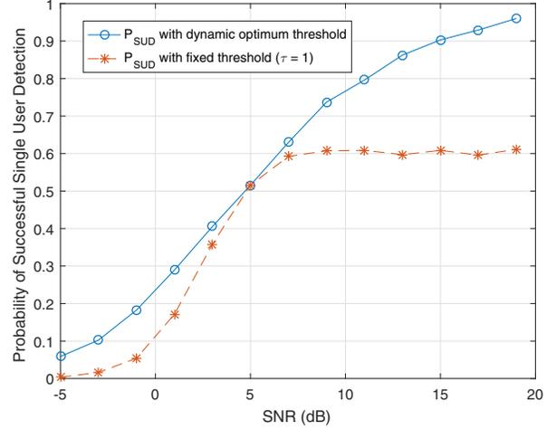
Fig. 5. Single user detection performance for the dynamic versus fixed detection threshold settings
