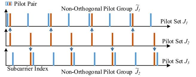
Fig. 2. Design of non-orthogonal pilot codes from orthogonal pilot sets
