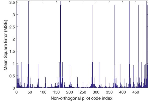
Fig. 1. Channel estimation performance of different non-orthogonal pilot codes from the existing design (SNR=0 dB)
