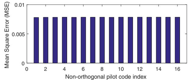
Fig. 4. Channel estimation performance of the proposed non-orthogonal pilot codes within a pilot group (SNR=0 dB)
