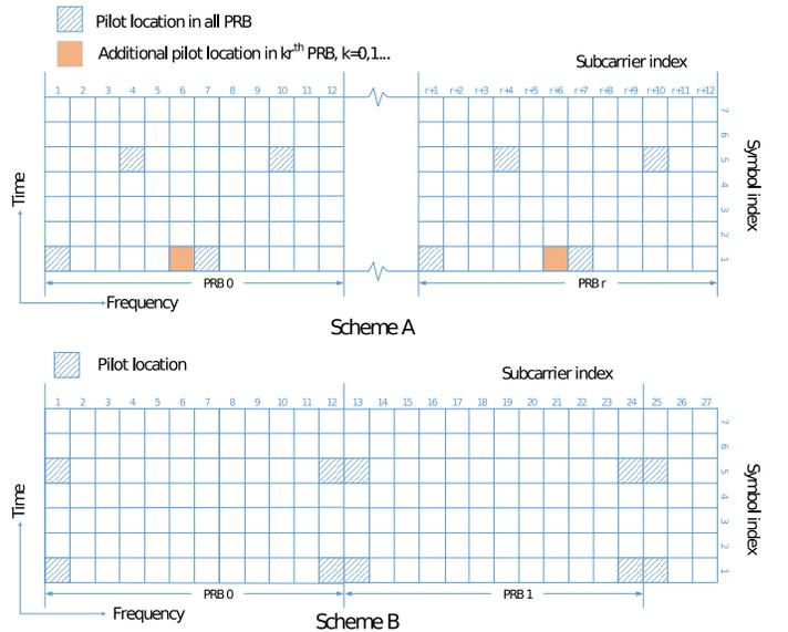
Fig. 7. Proposed pilot Scheme A and Scheme B for the fractional bandwidth allocation
