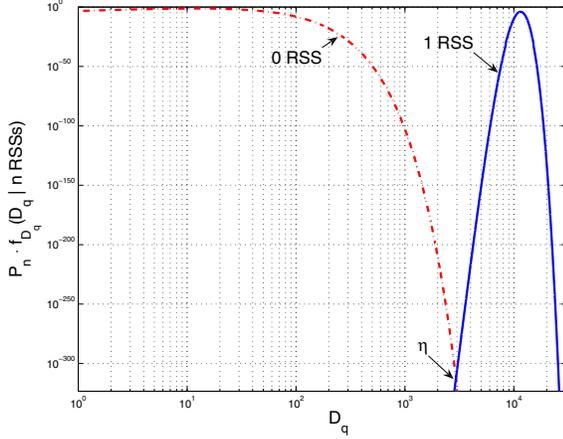
Fig. 1. The PDFs of the ranging code detection decision variable
