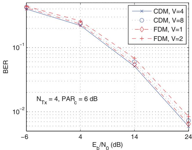
Fig. 3. BER performance comparison among different training structures of the FD design with  $\text{PAR}_c = 6$  dB and  $N_{T_x} = 4$ .
