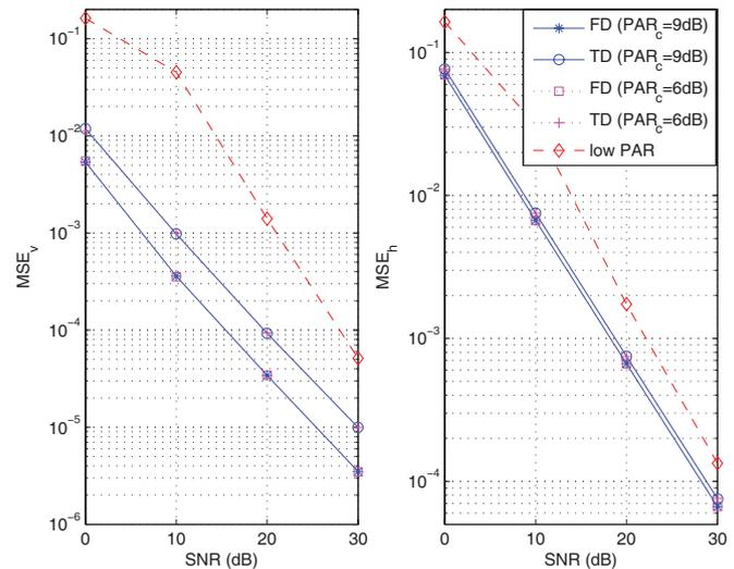
Fig. 4. Estimation performance comparison between the low PAR design and the proposed designs in an OFDM system with  $N_{T_x} = 4$  transmit antennas (FD design is based on the CDM structure with  $V = 4$ ).
