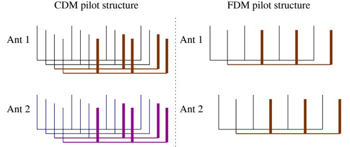
Fig. 1. An illustration of the proposed FD training design for a 16 subcarriers OFDM system with 2 transmit antennas in 4-tap channels. In the CDM structure,  $V = 4$  and  $\lambda = 5$ . In the FDM structure,  $V = 2$  and  $\lambda = 3$ . The pilots in thicker lines denote the modified pilots based on Newman's sequences.
