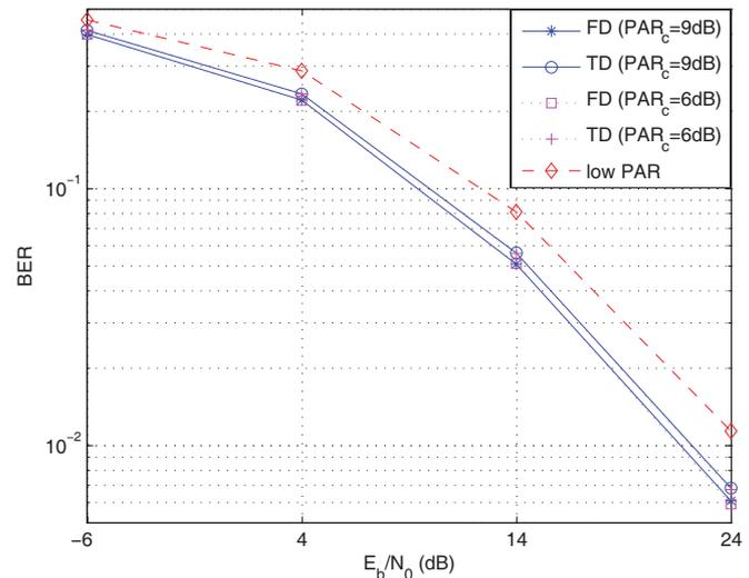
Fig. 5. BER performance comparison between the low PAR design and the proposed designs in an OFDM system with  $N_{T_x} = 4$  transmit antennas (FD design is based on the CDM structure with  $V = 4$ ).
