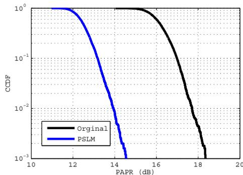
Fig. 8. PAPR characteristics of the proposed schemes in DL OFDM with 3 non-contiguous CCs and 16-QAM modulation, obtained by 5000 iterations
