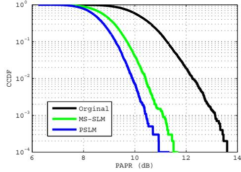
Fig. 5. PAPR characteristics of the proposed schemes with the optimization of 3 symbols in UL SC-FDMA with 16-QAM modulation, obtained by 10,000 iterations.
