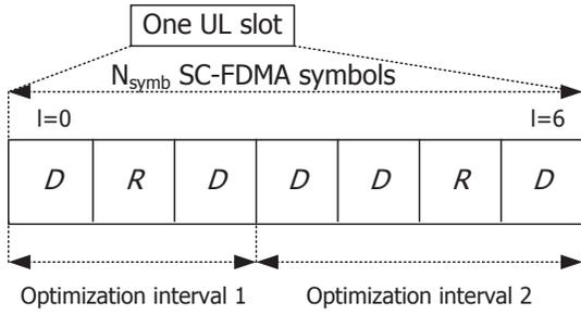
Fig. 2. One UL SC-FDMA time slot where  $D$  and  $R$  refer to data and reference symbol, respectively.
