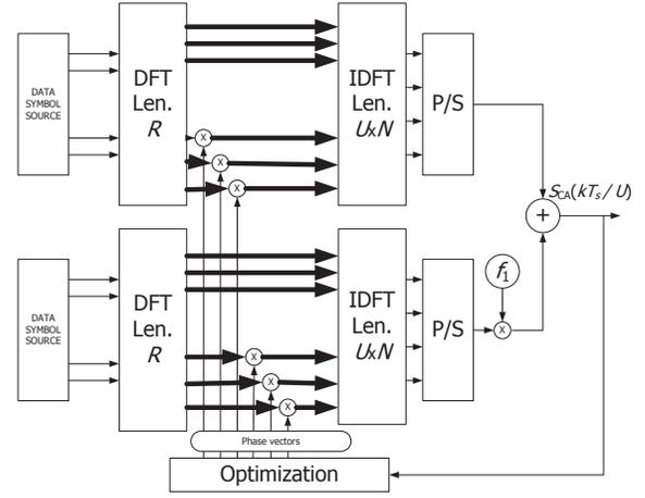
Fig. 3. Block diagram of the proposed method in UL scenario with 2 CCs. PAPR optimization is typically done in all discrete-time domain and in this case a larger IDFT size (where  $U$  is the oversampling factor) should be used.
