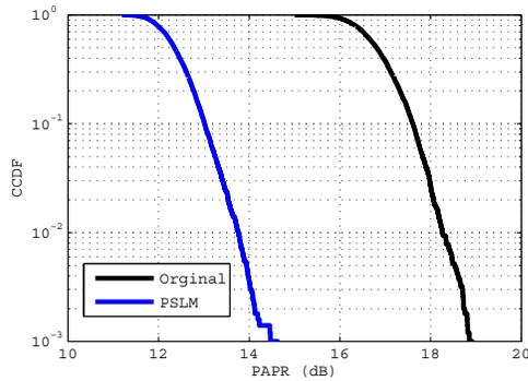
Fig. 7. PAPR characteristics of the proposed schemes in DL OFDM with 3 contiguous CCs and 16-QAM modulation, obtained by 5000 iterations
