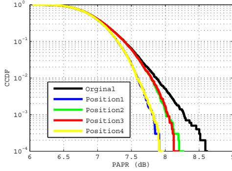
Fig. 4. Effect of group selection in UL SC-FDMA with QPSK modulation, obtained by 10,000 iterations.
