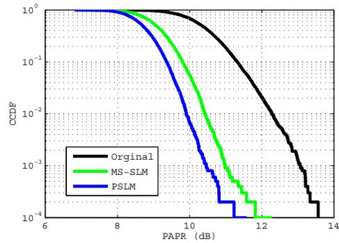
Fig. 6. PAPR characteristics of the proposed schemes with the optimization interval of 4 symbols in UL SC-FDMA, 16-QAM modulation, obtained by 10,000 iterations.
