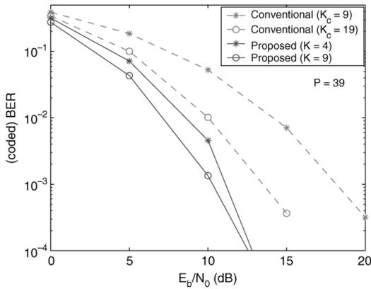
Fig. 7. Coded BER performance obtained with different training structures (rate-1/2 convolutional code).
