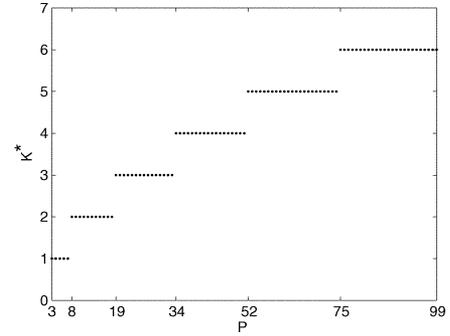
Fig. 4. Optimal value of  $K$  versus  $P$  for the optimal training structure containing  $(2K + 2)$  subblocks within the block length of  $P + 1$  subblocks. (The plot is continuous from the right, e.g., at  $P = 34$ ,  $K^* = 4$ .)
