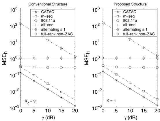
Fig. 11. Channel estimation MSE of different training subblock signals in a multipath Rayleigh fading channel.
