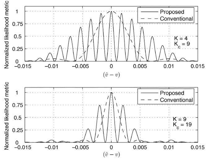
Fig. 18. Normalized likelihood metric of frequency offset estimation for the proposed training structure and the conventional structure using the same system resource (i.e.,  $K_c = 2K + 1$ ).
