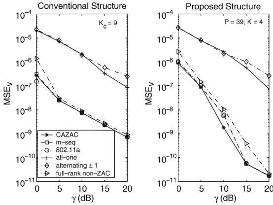
Fig. 10. Normalized frequency offset estimation MSE of different training subblock signals in a multipath Rayleigh fading channel.
