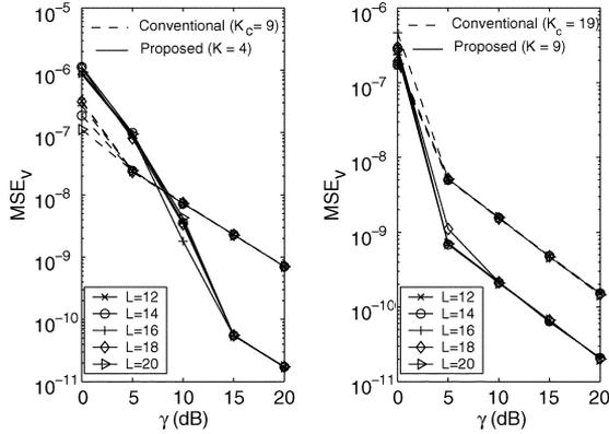
Fig. 14. Normalized frequency offset estimation MSE of several training signals with mismatched  $L$  values in a multipath Rayleigh fading channel (The design value for  $L$  is 16.)
