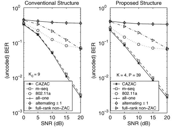
Fig. 12. Uncoded BER performance of different training subblock signals in a multipath Rayleigh fading channel.
