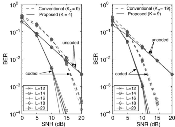
Fig. 16. Uncoded BER performance of different training signal structures with mismatched  $L$  values in a multipath Rayleigh fading channel (the design value for  $L$  is 16.)
