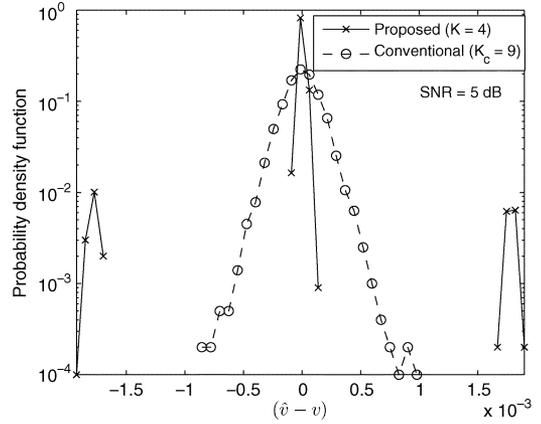
Fig. 8. PDF (obtained by simulation) of the normalized frequency offset estimation error for different training structures.
