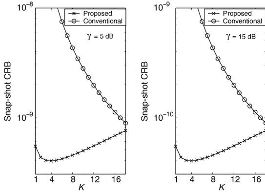
Fig. 3. Snapshot CRB for different periodic training structures as a function of  $K$  (for the conventional structure,  $K_c = 2K + 1$ ).
