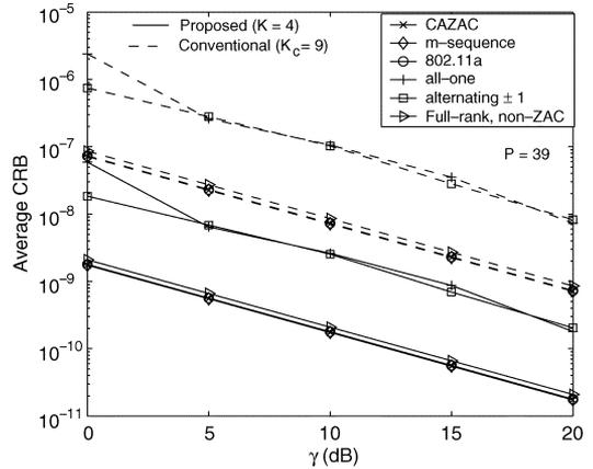
Fig. 9. Average CRB of the normalized frequency offset estimation for different training structures with different subblock signals in a multipath Rayleigh fading channel.
