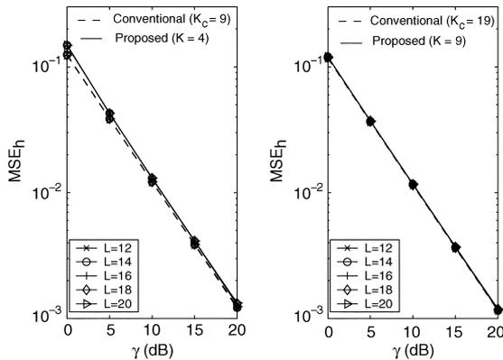
Fig. 15. Channel estimation MSE of different training subblock signals with mismatched  $L$  values in a multipath Rayleigh fading channel (the design value for  $L$  is 16.)
