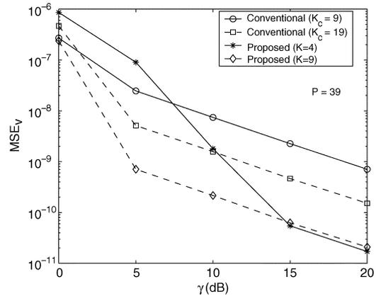
Fig. 5. Normalized frequency offset estimation MSE for different periodic training structures.
