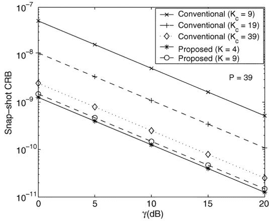
Fig. 2. Snapshot CRB of the normalized frequency offset estimation with different periodic training structures.
