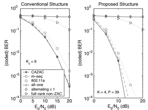
Fig. 13. Coded BER performance of different training subblock signals in a multipath Rayleigh fading channel (rate-1/2 convolutional code).
