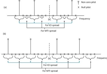
Fig. 3. The basic design approach for estimating effective channel gains, ICI and MTI coefficients. (a)  $\kappa = 1$  and  $\iota = 0$ , (b)  $\kappa = 1$  and  $\iota = 1$
