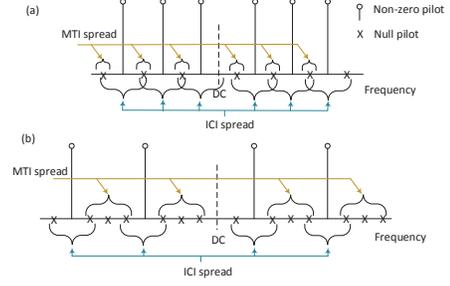
Fig. 2. The basic design approach for estimating main diagonal elements of  $\mathbf{Q}_{ij}$ . (a)  $\kappa = 1$  and  $\iota = 0$ , (b)  $\kappa = 1$  and  $\iota = 1$
