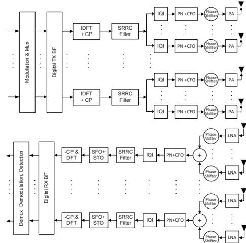
Fig. 1. Downlink MIMO-OFDM signal model block diagram with RF impairments. (SRRC = square-root raised cosine filter, PA = power amplifier, LNA = low-noise amplifier, SFO = sampling frequency offset, STO = sampling time offset, BF = beam-forming, CP = cyclic prefix)
