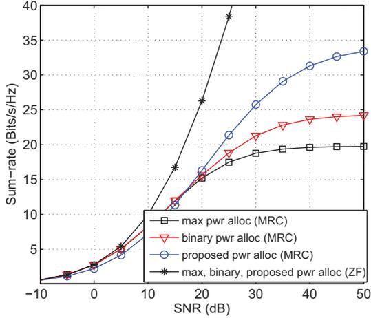
Fig. 1. Power allocation performance (sum-rate versus maximum Tx SNR) for MRC and ZF receiver with imperfect CSI.
