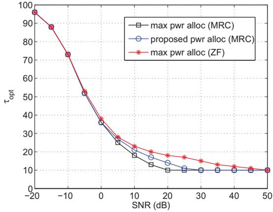
Fig. 2. The optimal number of pilot symbols versus maximum Tx SNR for MRC and ZF receivers with power allocation.
