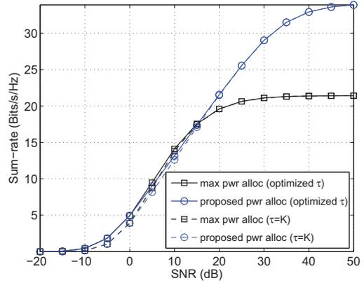
Fig. 3. Comparison between optimized  $\tau$  and  $\tau = K$  in terms of sum-rate versus maximum Tx SNR for MRC receiver.
