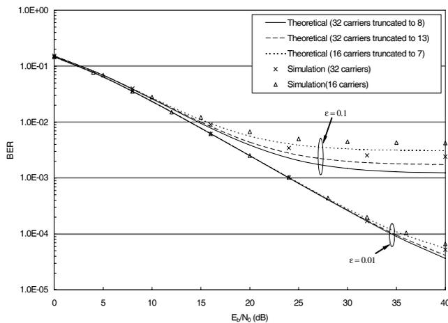
Fig. 5. BER performance with ICI truncation over frequency selective Rayleigh fading channel having  $L = 5$ .
