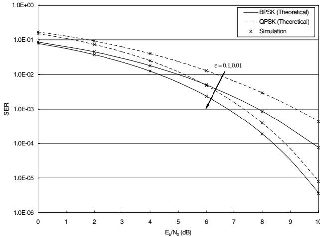
Fig. 1. Probability of symbol error for BPSK/QPSK over AWGN channel with  $N = 8$ .
