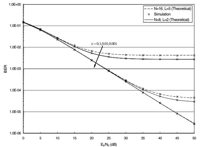
Fig. 4. BER for BPSK over frequency selective Rayleigh fading channel.
