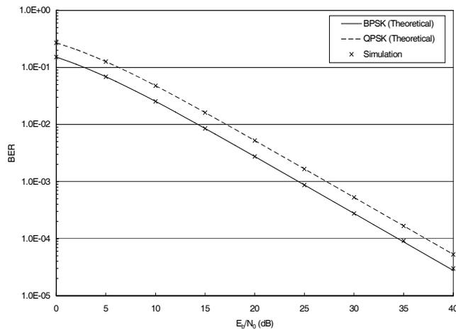
Fig. 2. Probability of symbol error for BPSK/QPSK over Rayleigh flat fading channel with  $N = 8$ ,  $\epsilon = 0.1$  and  $\sigma_R^2 = 0.5$ .
