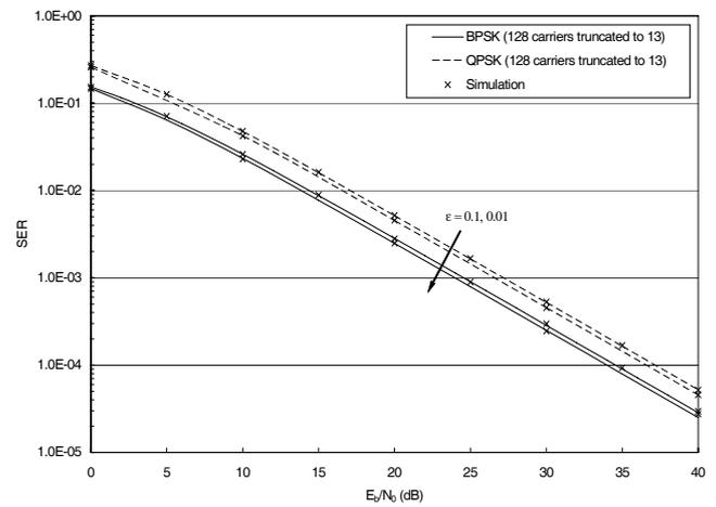
Fig. 3. Approximate performance of BPSK/QPSK over Rayleigh flat fading channel with  $N = 128$  and  $\sigma_R^2 = 0.5$ .
