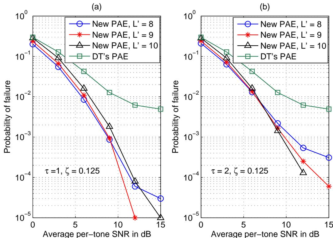
Figure 7. Performance comparison between the proposed PAE and DT's PAE in the presence of timing and sampling offsets at  $v = 4$ .
