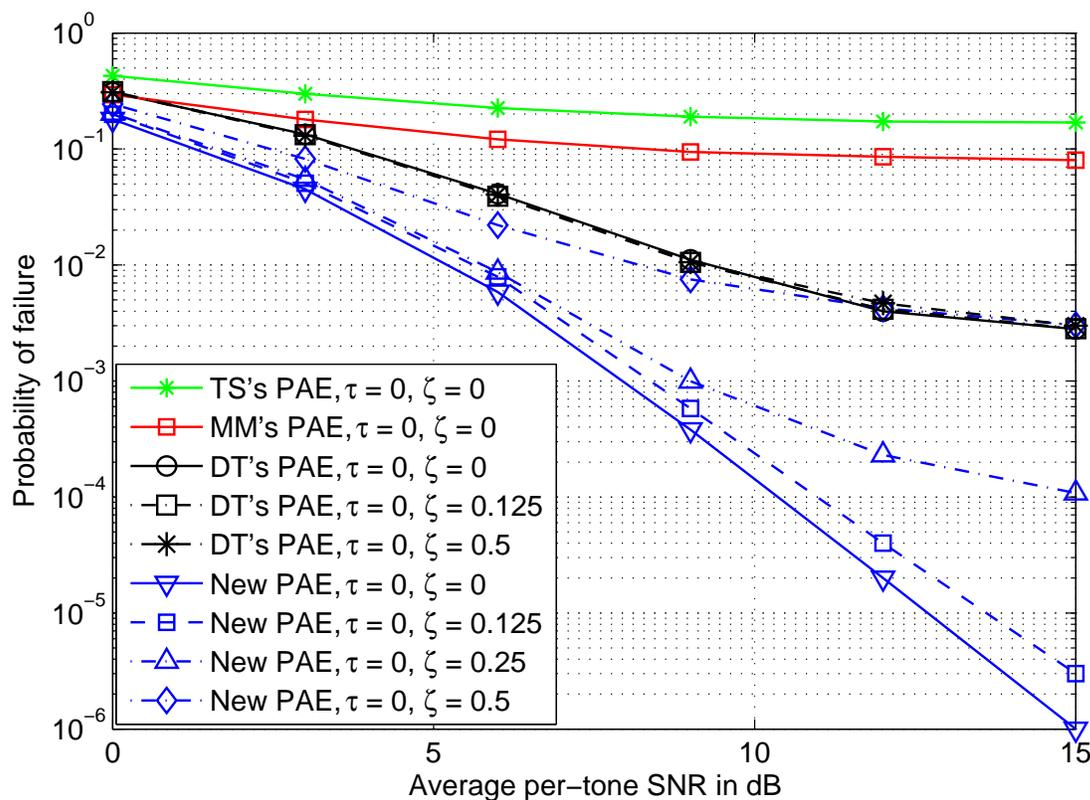
Figure 5. Performance comparison of different ICFO estimators under the accurate signal model with  $v = 4$
