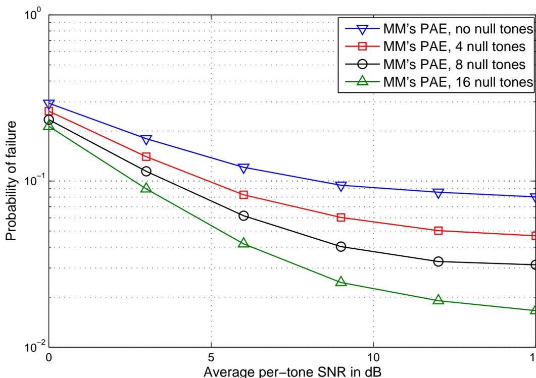
Figure 1. MM's PAE with different numbers of null tones at the band edge (perfect synchronization, 16 pilot tones,  $v = 4$ )
