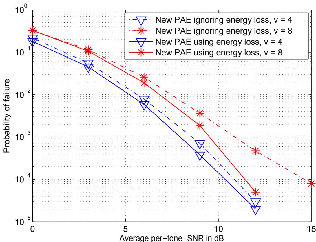
Figure 6. ICFO estimation performances of the new PAE using versus ignoring the energy loss information under the accurate signal model.
