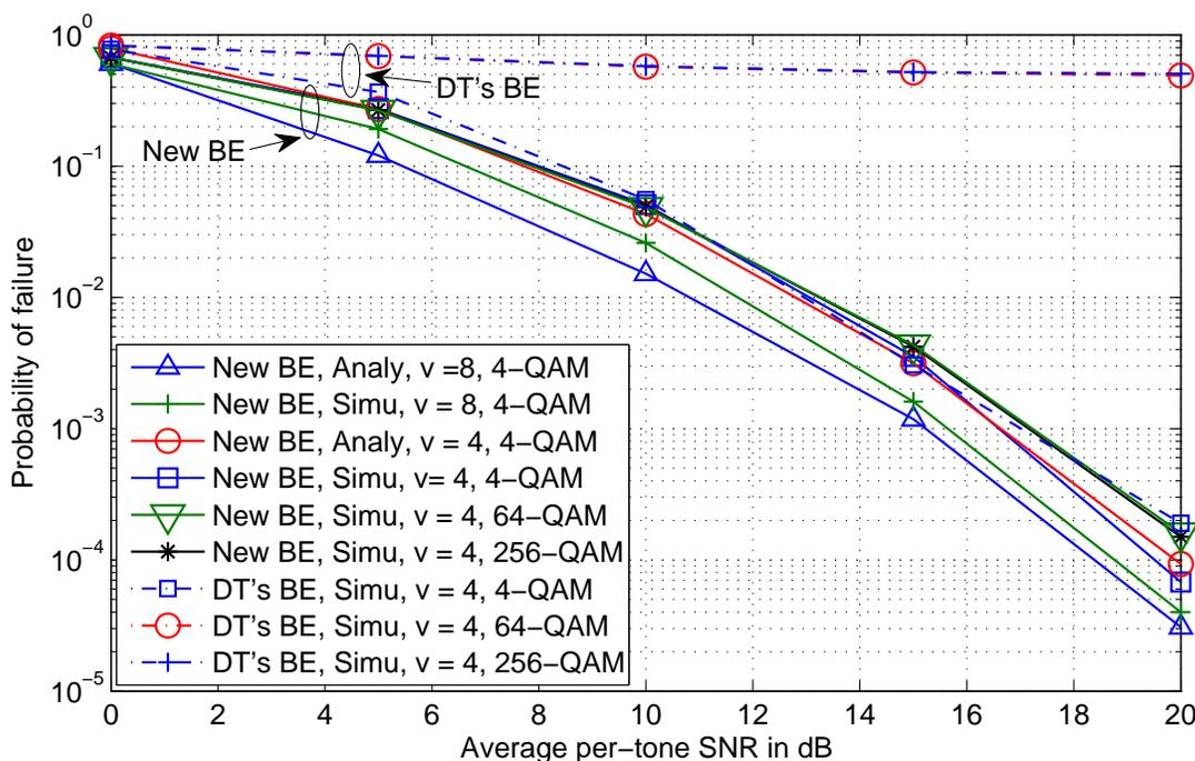
Figure 11. Effects of QAM order on the performance of the new BE and DT's BE, and comparison between the simulation and approximate analytical results of the new BE ( $\tau = 0$ , uniform random  $\zeta \in [-0.125, 0.125]$ ).
