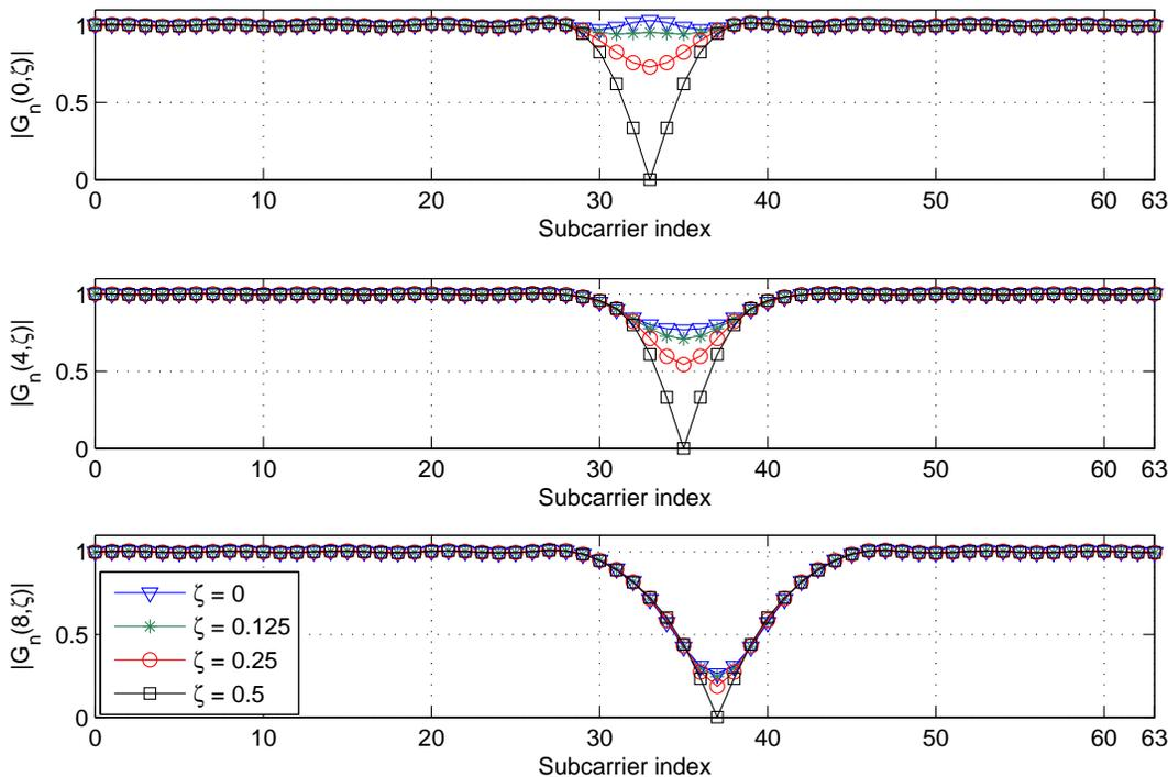
Figure 3. Effects of CFO and sampling offset on the equivalent filter gain: Top ( $v = 0$ ), Middle ( $v = 4$ ), Bottom ( $v = 8$ )
