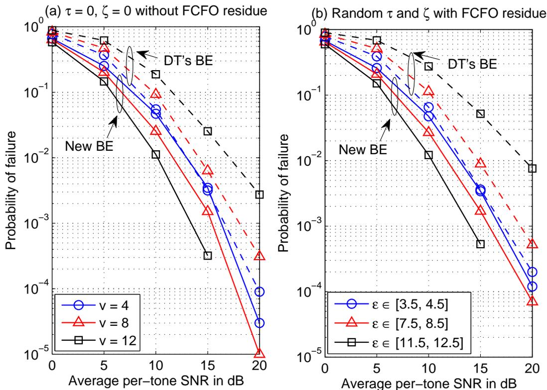
Figure 10. Effects of different CFO values on the estimation performances of the new BE and DT's BE
