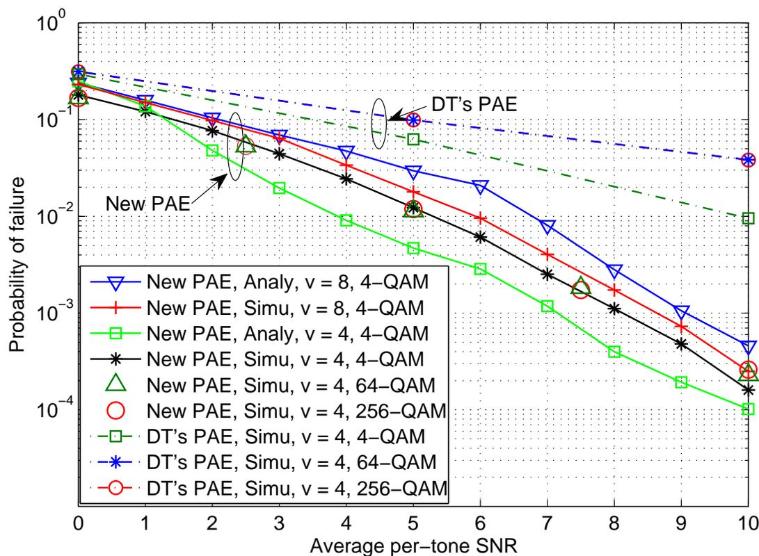
Figure 9. Effects of QAM order on the performance of the new PAE and DT's PAE, and comparison between the simulation and approximate analytical results of the new PAE ( $\tau = 0$ , uniform random  $\zeta \in [-0.125, 0.125]$ ).
