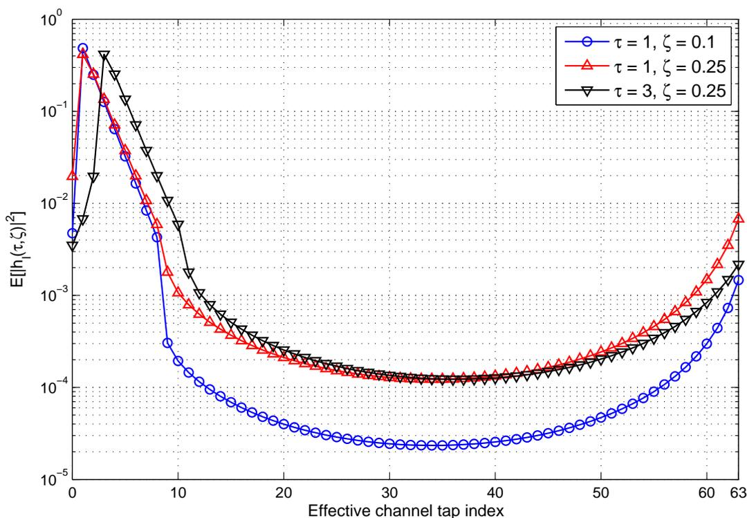
Figure 2. Impact of timing and sampling offsets on the effective wireless channel taps
