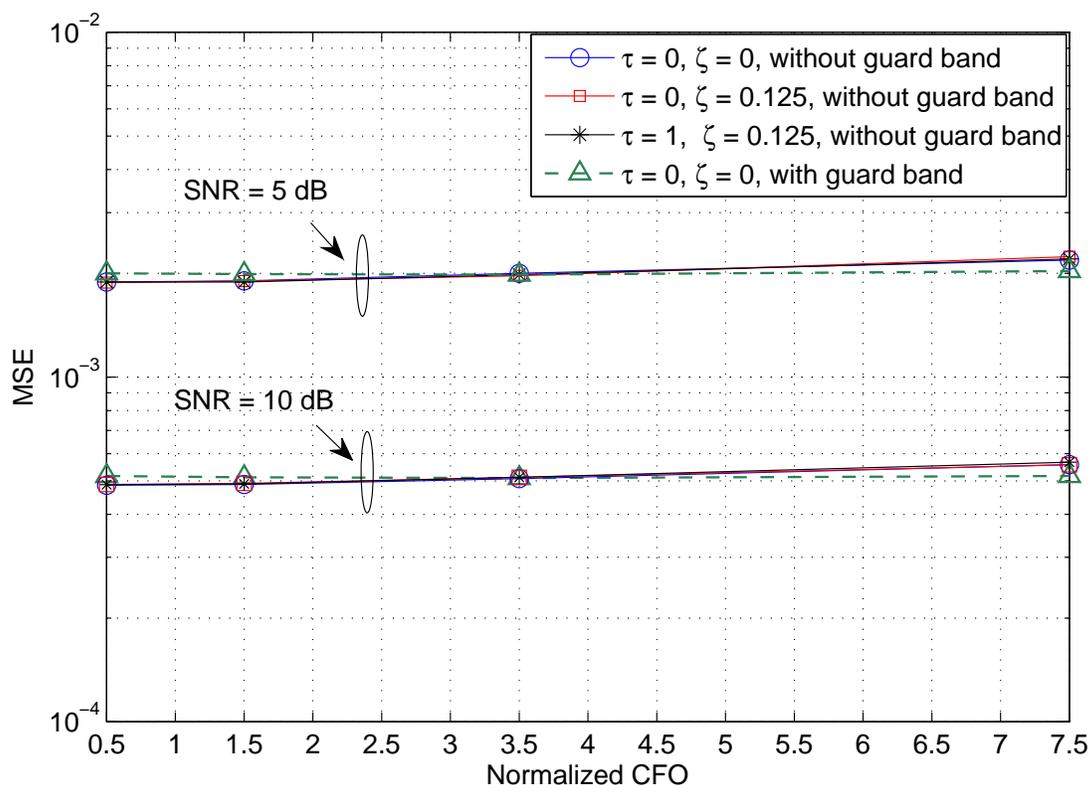
Figure 4. FCFO estimation performance of a correlation-based estimator under the accurate signal model
