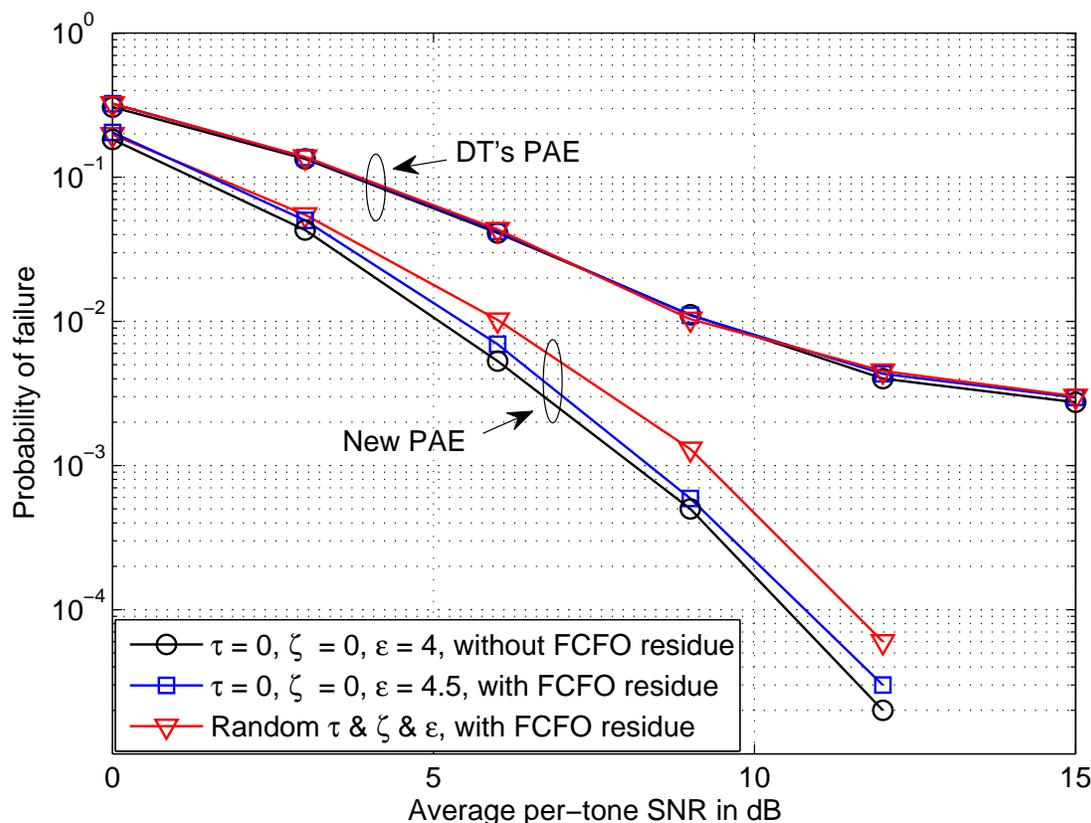
Figure 8. Effect of residual FCFO on ICFO estimation performance of the new PAE and DT's PAE.
