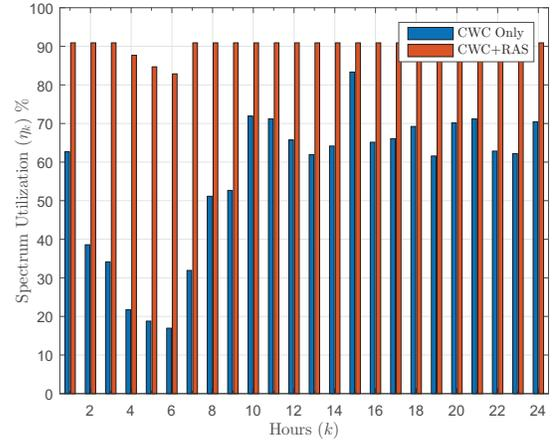
Fig. 7. Spectrum utilization comparison between the CWC only allocation and the shared allocation
