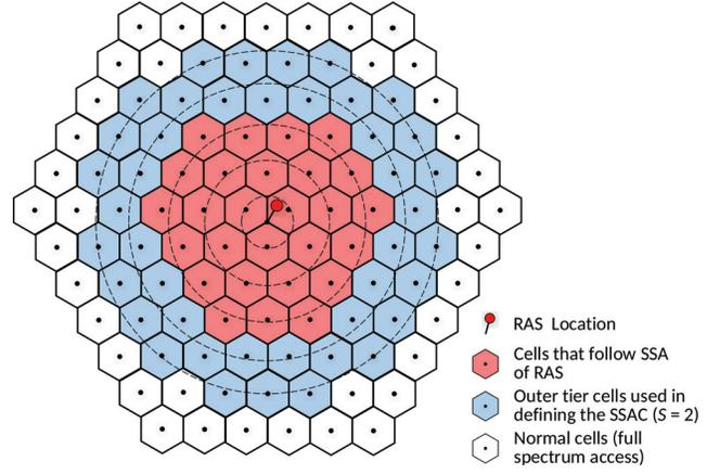
Fig. 1. Tiers of CWC cell rings around an RAS receiver
