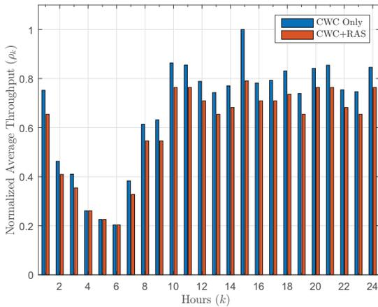
Fig. 6. CWC average throughput comparison between the CWC only allocation and the shared allocation
