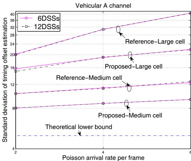
Fig. 9. Timing offset estimation performance in vehicular A channel.
