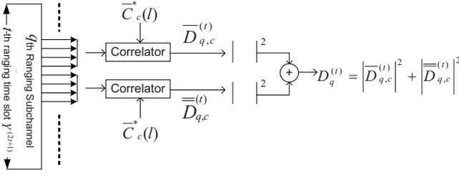
Fig. 2. The block diagram of the proposed ranging signal detector.
