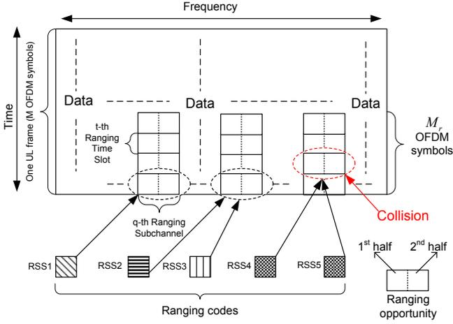
Fig. 1. Illustration of ranging resource structuring.
