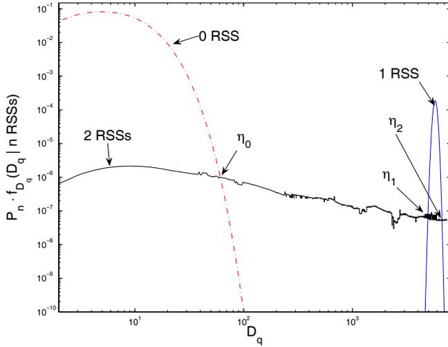
Fig. 3. The PDFs of the ranging code detection decision variable.
