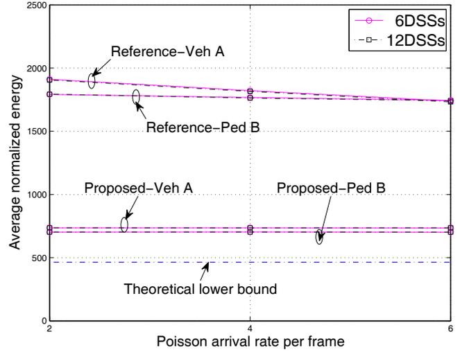
Fig. 10. Average normalized ranging transmission energy per frame.
