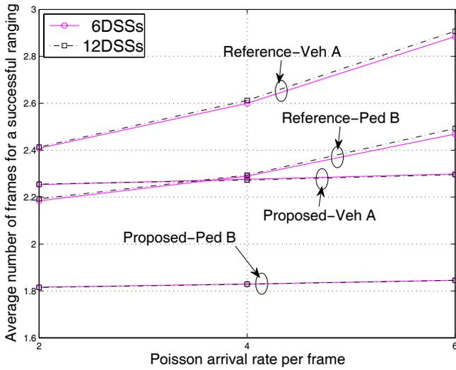
Fig. 7. Average number of ranging frames required for a successful ranging.
