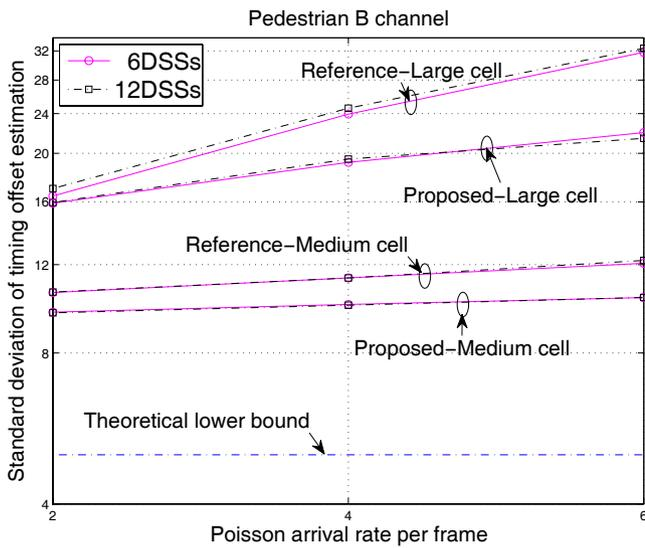
Fig. 8. Timing offset estimation performance in pedestrian B channel.
