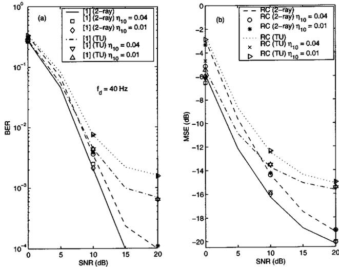
Fig. 9. Performance of the channel estimation methods with adaptive significant tap selection ( $J_m = 7$ ,  $\alpha = 4$ ) in two-ray and TU channels with delay spread of  $1.06 \mu\text{s}$ , and the Doppler frequency of 40 Hz for OFDM with 4-PSK, 16 states space-time code.
