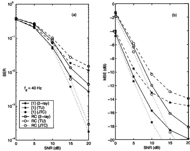
Fig. 8. Performance of the channel estimation methods in OFDM with 16-QAM, 16 states space-time code. The rms delay spread is  $1.06 \mu\text{s}$  for two-ray and TU, 34.8 ns for JTC, the Doppler frequency is 40 Hz.
