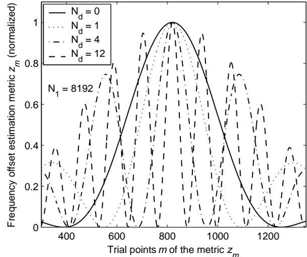
Fig. 6. The frequency offset estimation metric trajectories of the modified training structure with different values of  $N_d$
