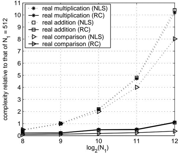
Fig. 3. The estimation complexities of the NLS and RC methods ( $N_2 N_c = 2N_1$ ) relative to that of the NLS with  $N_1 = 512$
