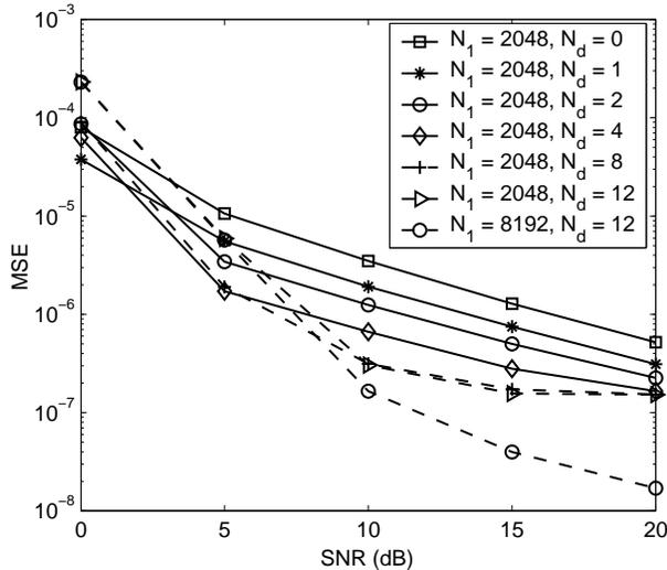
Fig. 5. The estimation MSE performance obtained with the existing training structure ( $N_d = 0$ ) and the proposed modified training structure ( $N_d \neq 0$ )
