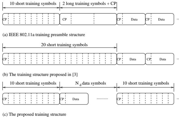
Fig. 1. The training structures for OFDM-based WLANs
