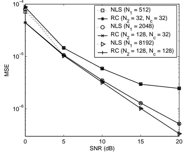
Fig. 4. The comparison of estimation MSE performance of the proposed RC method and the NLS method
