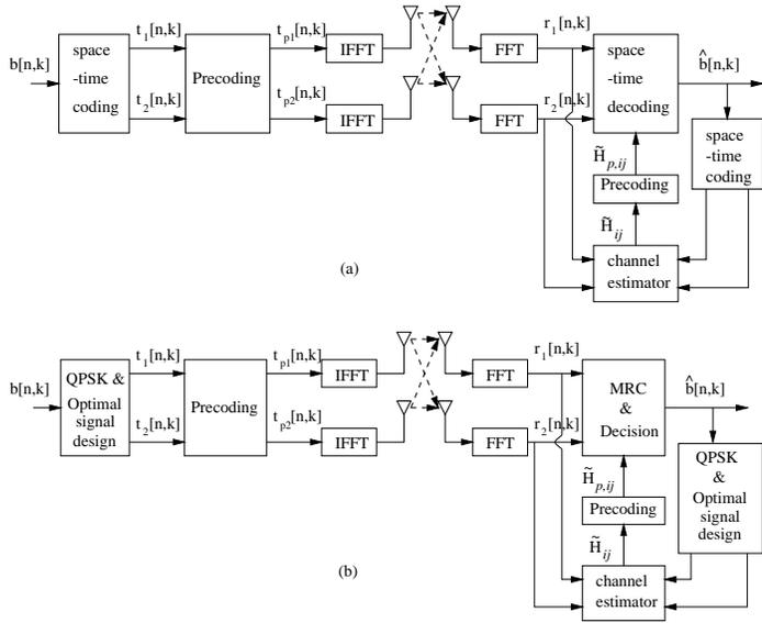
Fig. 1. Proposed reduced complexity channel estimation for OFDM systems with transmit diversity in two schemes: (a) 1<sup>st</sup> scheme using space-time coding, (b) 2<sup>nd</sup> scheme using optimal signal design and MRC reception
