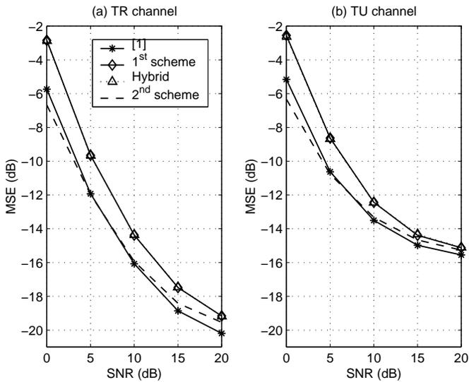
Fig. 2. Channel estimation MSE performances for OFDM systems with transmit diversity: (a) TR channel and (b) GSM-TU channel.
