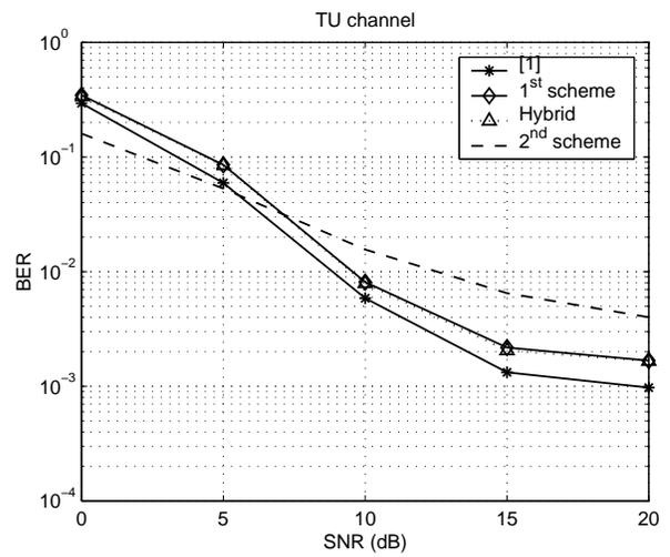
Fig. 4. BER performances of OFDM systems with transmit diversity using different channel estimation methods in GSM-TU channel.
