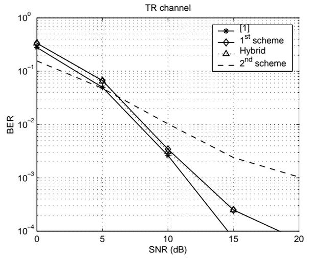
Fig. 3. BER performances of OFDM systems with transmit diversity using different channel estimation methods in TR channel.
