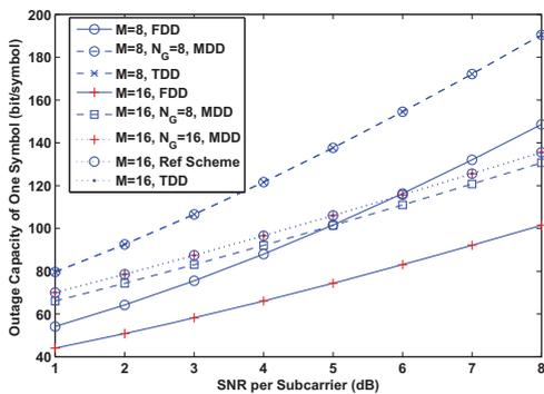
Fig. 5. Comparison of outage capacity per symbol for different duplexing schemes at  $P_{out} = 10^{-4}$  (the effects of ICI and guard intervals are excluded)
