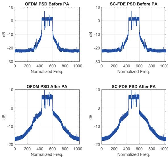
Fig. 6. The PSD of OFDM and SC-FDE TX signals before and after the amplifier with 4dB backoff for system 3.
