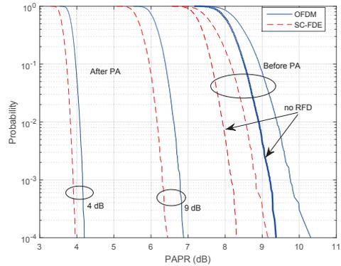
Fig. 4. The CCDF of the PAPR of OFDM and SC-FDE TX signals before and after the power amplifier for system 3.
