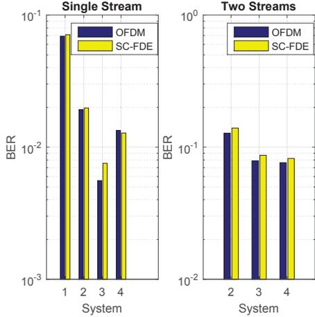
Fig. 2. Un-coded BER of systems with one and two data streams in DL
