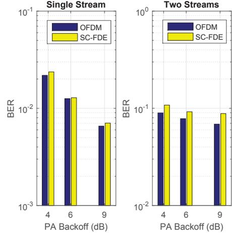
Fig. 3. Effects of PA backoff on un-coded BER of system 3 with one and two data streams in UL
