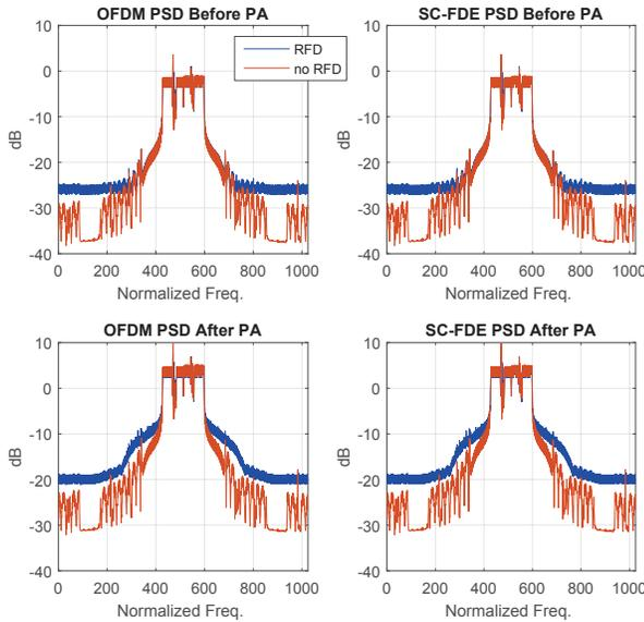
Fig. 5. The PSD of OFDM and SC-FDE TX signals before and after the amplifier with 9 dB backoff for system 3.
