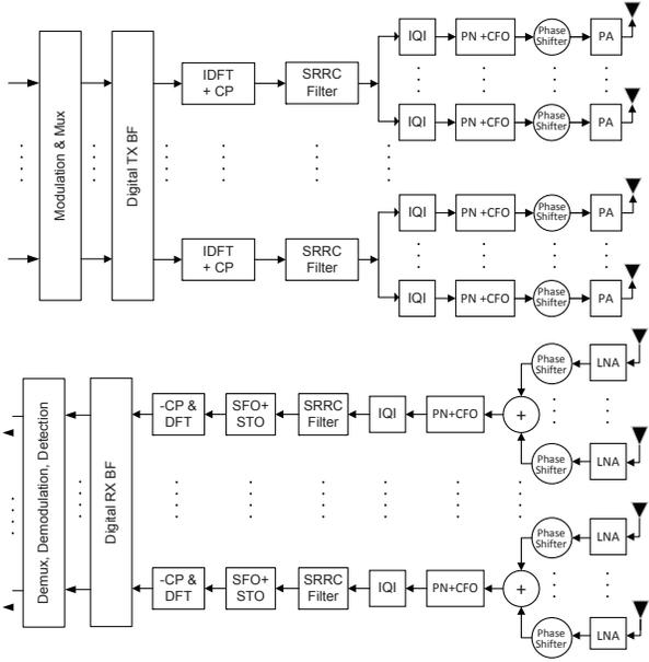
Fig. 1. MIMO-OFDM signal model block diagram with RF impairments. (SRRC = square-root raised cosine filter, PA = power amplifier, LNA = low-noise amplifier, SFO = sampling frequency offset, STO = sampling time offset, BF = beam-forming, CP = cyclic prefix)
