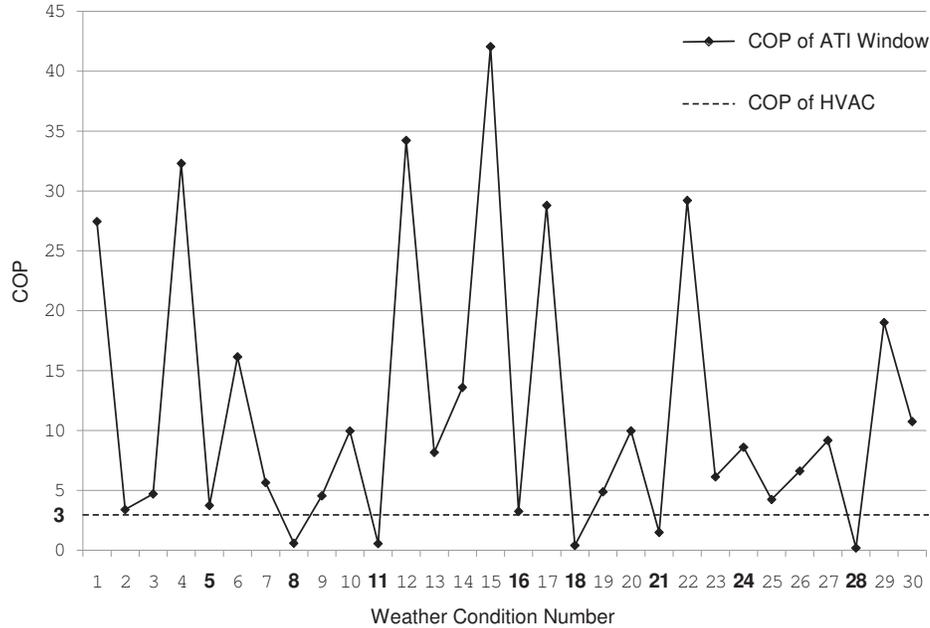
Figure 6. Values of  $COP_{ATI}$  under Different Weather Conditions
