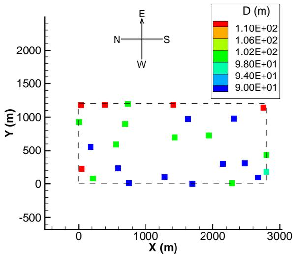
(c) Showing the rotor-diameters of individual turbines
