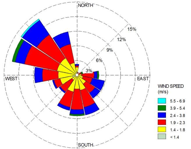
**FIGURE 3.** Windrose diagram for Baker station, ND (Years 2000-2009)
