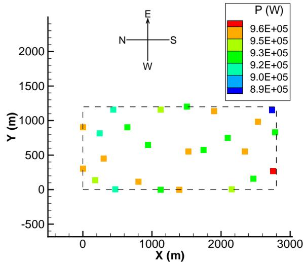
**FIGURE 5.** Layout of the optimized wind farm for Case 1
