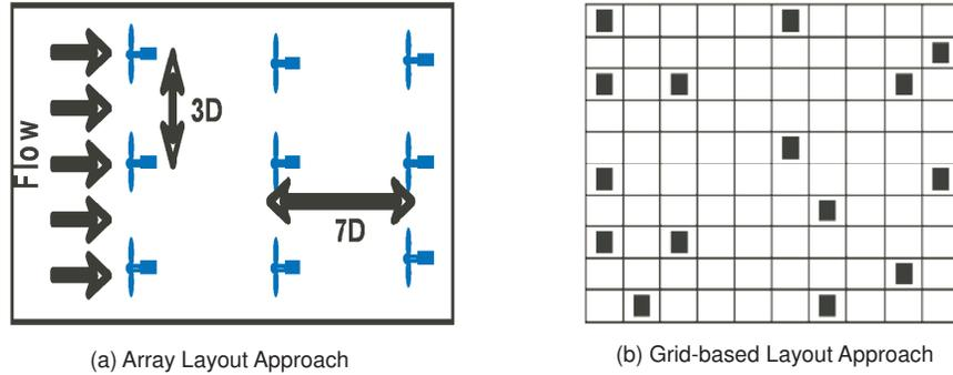
**FIGURE 1.** Existing approaches in wind farm optimization: (a) Array layout approach, and (b) Grid-based approach
