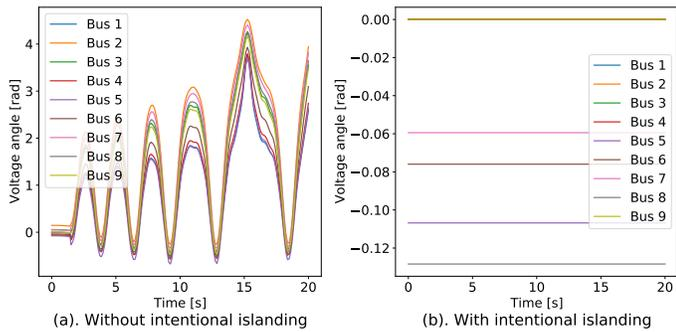
**FIGURE 8: The dynamic response of the voltage angle at all buses of the IEEE 9-bus system after disruptions, with and without the intentional islanding operation**
