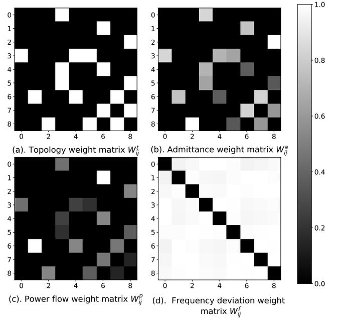
FIGURE 3: Four weight matrices constructed from the measurement data of the IEEE 9-bus system.
