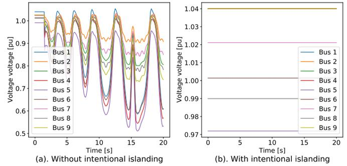
**FIGURE 7: The dynamic response of the voltage magnitude at all buses of the IEEE 9-bus system after disruptions, with and without the intentional islanding operation**
