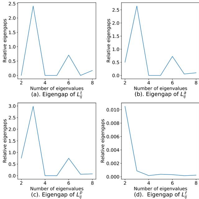
**FIGURE 4: The eigengap obtained from the four Laplacian matrices defined based on topology, admittance, power flow, and frequency deviation**
