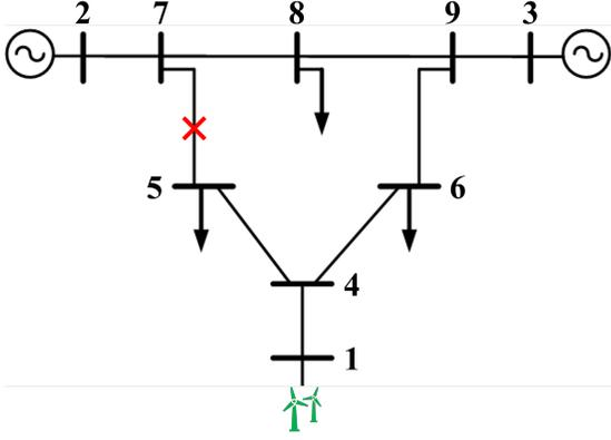
FIGURE 2: The one-line diagram of the IEEE-9 bus system, where the synchronous generator at bus 1 has been replaced by a wind farm (figure modified from [33]).
