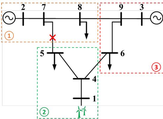
**FIGURE 6: The intentional islanding results for the IEEE 9-bus system based on the derived dendrogram (figure modified from [33])**
