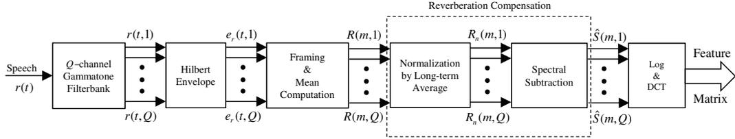
Fig. 1. Block diagram of the MHEC feature extraction framework. The symbols represent the output signals at each stage.
