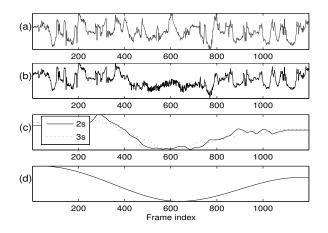
Figure 2: Time trajectory of the 2nd MFCC cepstral coefficient  $(C_2)$  for: (a) the clean speech, (b) degraded speech, (c) the block-wise mean computed using 2s and 3s sliding windows from the degraded speech  $C_2$  (d) summation of the residual and the last IMF generated from EMD computed from the degraded speech  $C_2$ .
