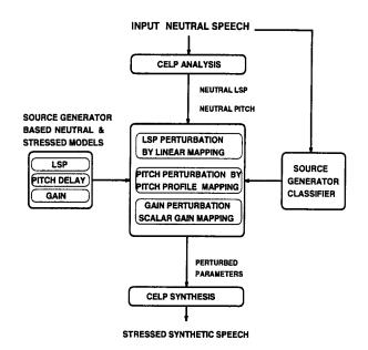
Figure 4: Flow graph for generating stressed synthetic speech via the CELP coder.
