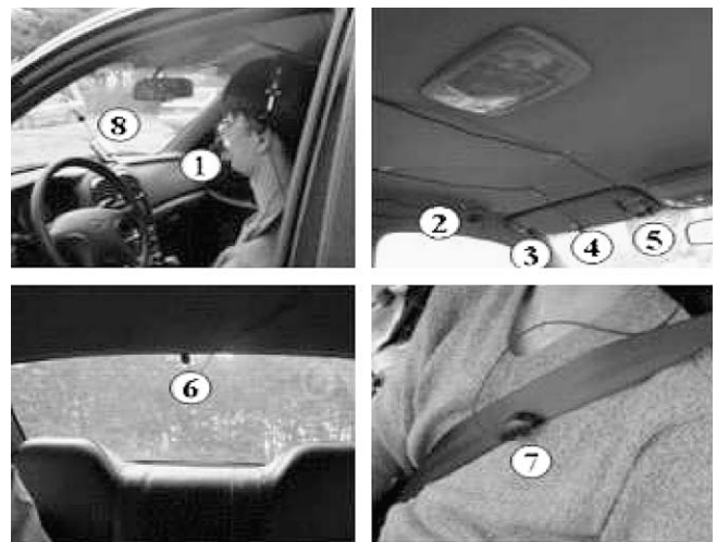
Fig. 6. The locations of microphones used for collecting the speech database Car01 under real car-driving condition.
