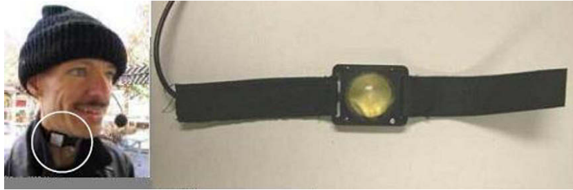
Fig. 2. The physiological sensor (PMIC) (on right) and its placement (left) around the neck near cycloid thyroid cartilage.
