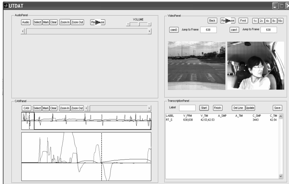
Figure 8 UTDAT multi-media data annotation tool, capable of cross-referencing and synchronisation of 2 video, 1 audio and CAN-Bus streams
