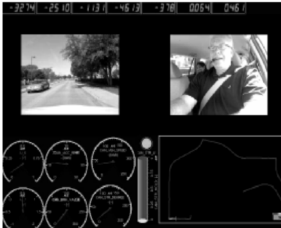
Figure 5 Data acquisition interface showing audio signals, video channels, CAN-Bus and GPS
