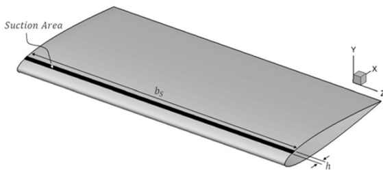
Fig. 4 NACA 0012 wing with suction slot
