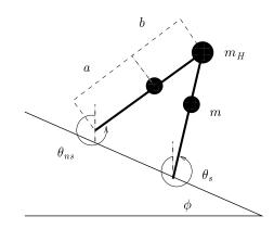
Consider a compass-gait biped with only a hip torque as a system of two-coupled pendula. Let the hip torque control be given as
