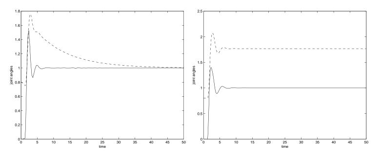
The new architecture (left) ensures convergence of the tracking error to zero even after an initial offset.
