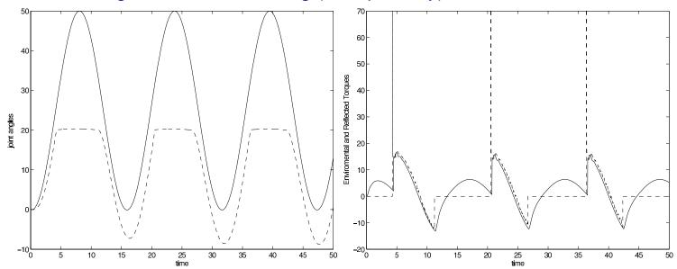
The master and the slave joint positions during contact with the environment(left).
