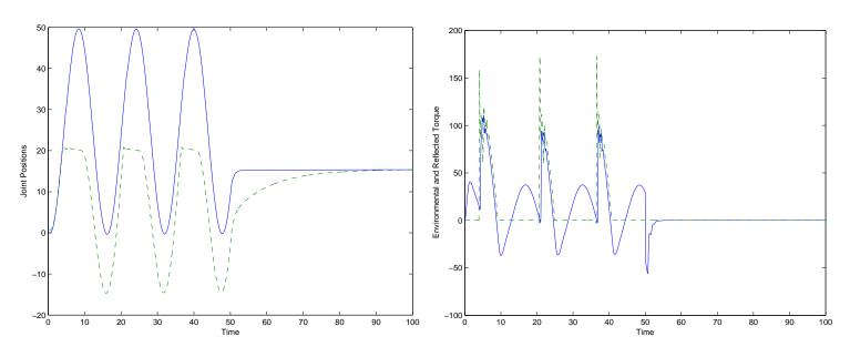
Blue shows the master position (left) and force (right) Green shows the slave position (left) and force (right)
