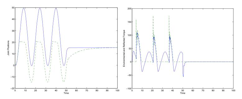
Blue shows the master position (left) and force (right) Green shows the slave position (left) and force (right)
