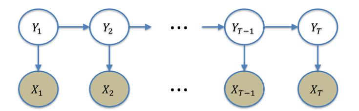
$$p(x_1, \dots, x_T, y_1, \dots, y_T) = p(y_1)p(x_1|y_1) \prod_{t=2} p(y_t|y_{t-1})p(x_t|y_t)$$
