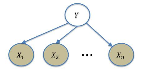
$$p(y, x_1, \dots, x_n) = p(y)p(x_1|y) \dots p(x_n|y)$$
