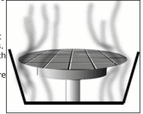
The slower rate of drying offers the advantage of increased film thickness uniformity across the substrates. The fluid dries out as it moves toward the edge of the substrate during the spin process. This can lead to radial thickness nonuniformities since the fluid viscosity changes with distance from the center of the substrate. By slowing the rate of drying, it is possible for the viscosity to remain more constant across the substrate.
